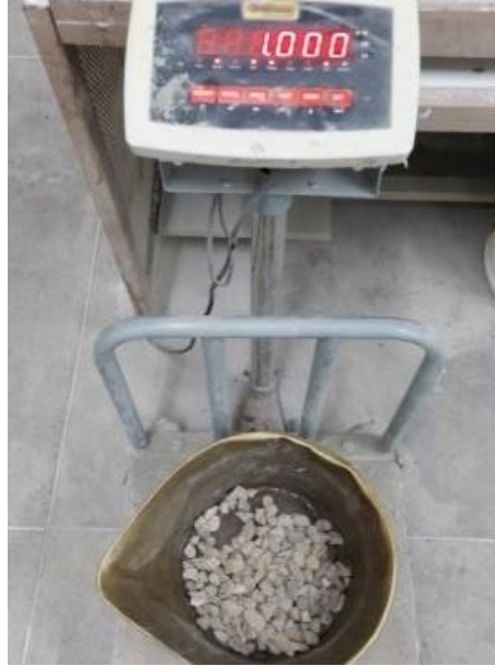
Figure 3.7: Weighing the Aggregates
