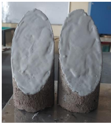
Figure 3.19: Application of Epoxy on the Specimen.
