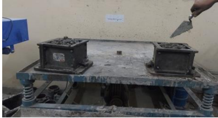
Fig. 3.13: Vibrating of Concrete
