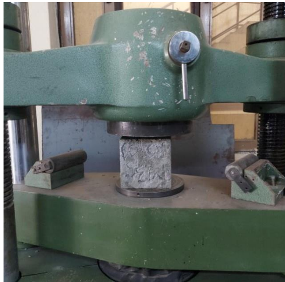
Fig. 3.14: Testing of the cubes
