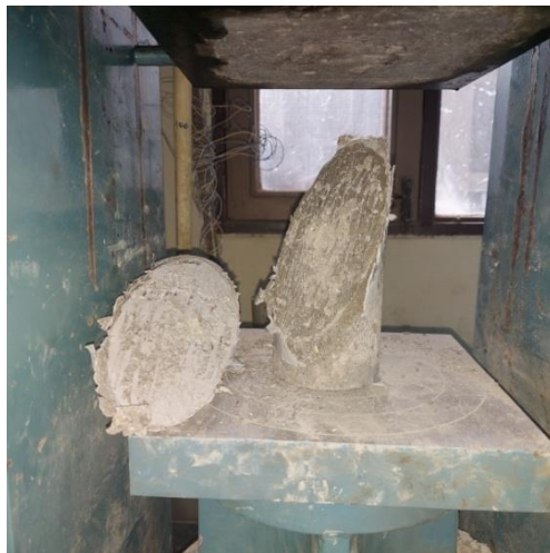
Figure 4.2: Failure of the Slant Surface
