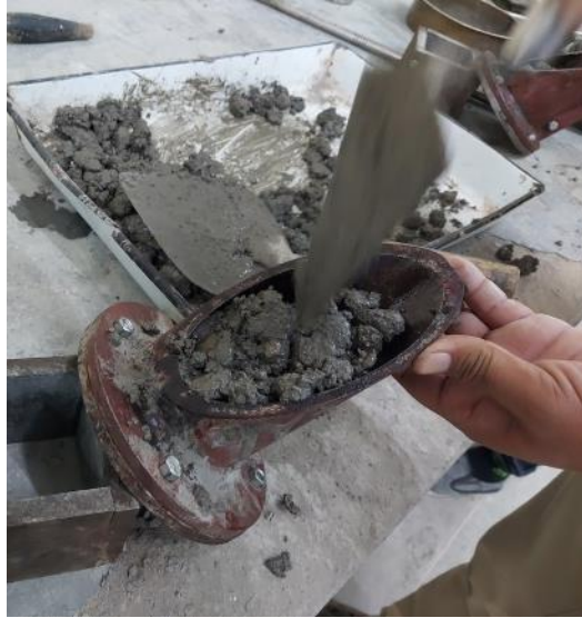
Figure 3.16: Casting of cylindrical specimen
