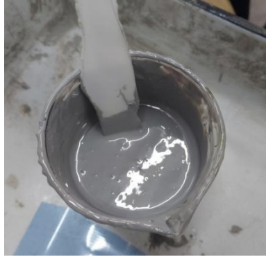
Figure 3.18: Mixing of Epoxy with the Hardener
