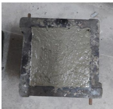
Fig. 3.12: Casting of M25
