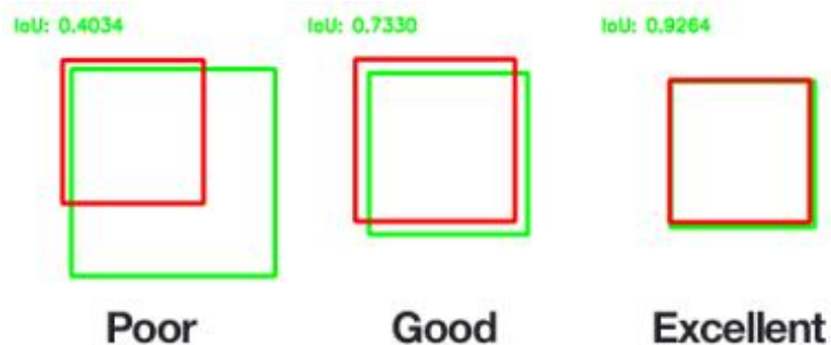
Figure 3.2: Example of computing IOU for various bounding boxes
