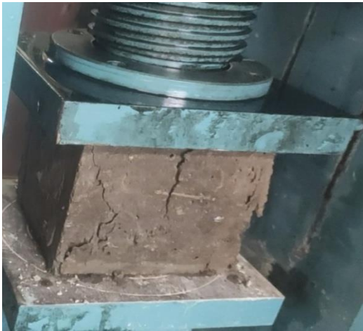
Fig 4.2 Compression testing of normal concrete.
