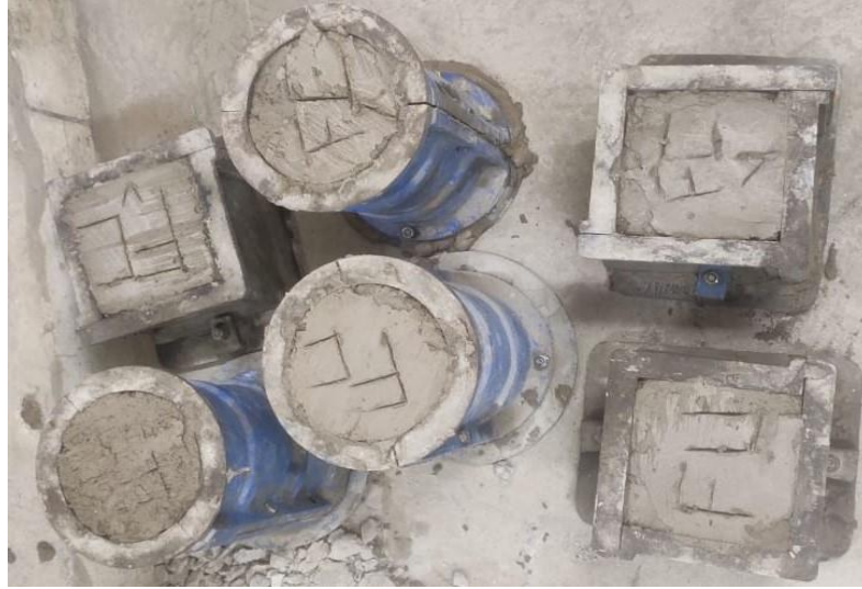
Fig 3.11 Casting of foamed concrete blocks
