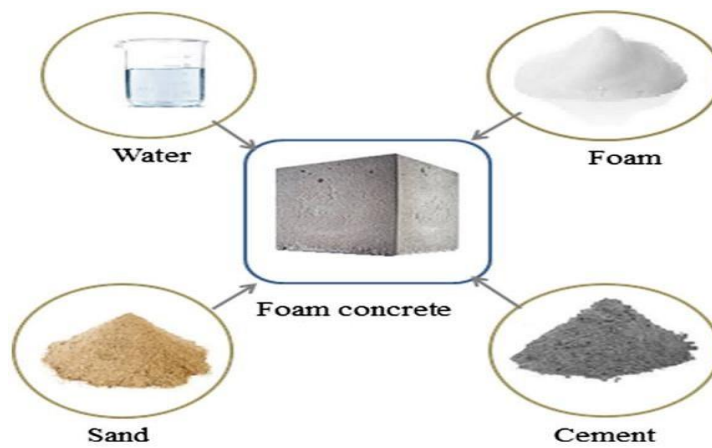
Fig 1.2 Constituents of foamed concrete [1]
