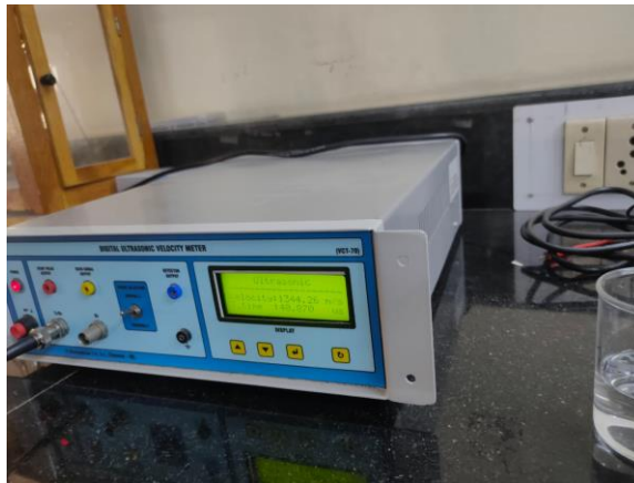
Figure 9: Shows pulse echo velocity meter
