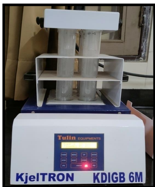
Fig 14 – KjelTRON digestion system
