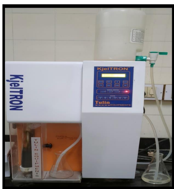
Fig 15- KjelTRON system for distillation
