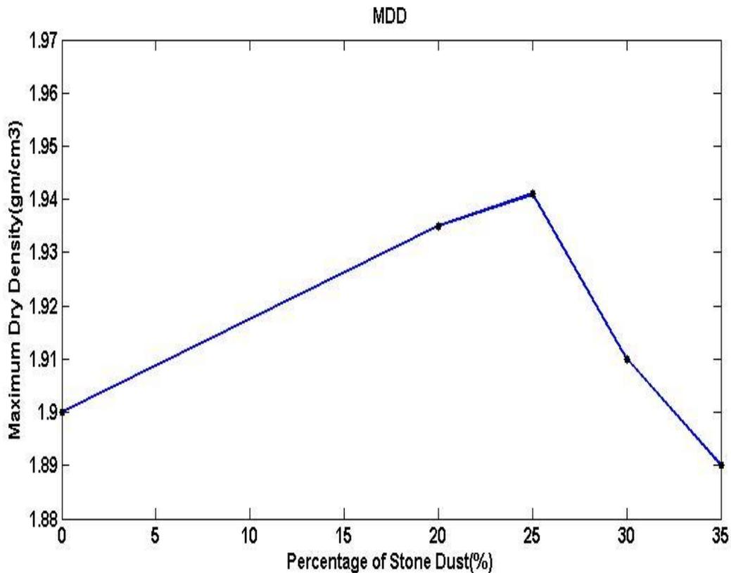
**Fig 20. Variation of maximum Dry density with % of stone dust**
