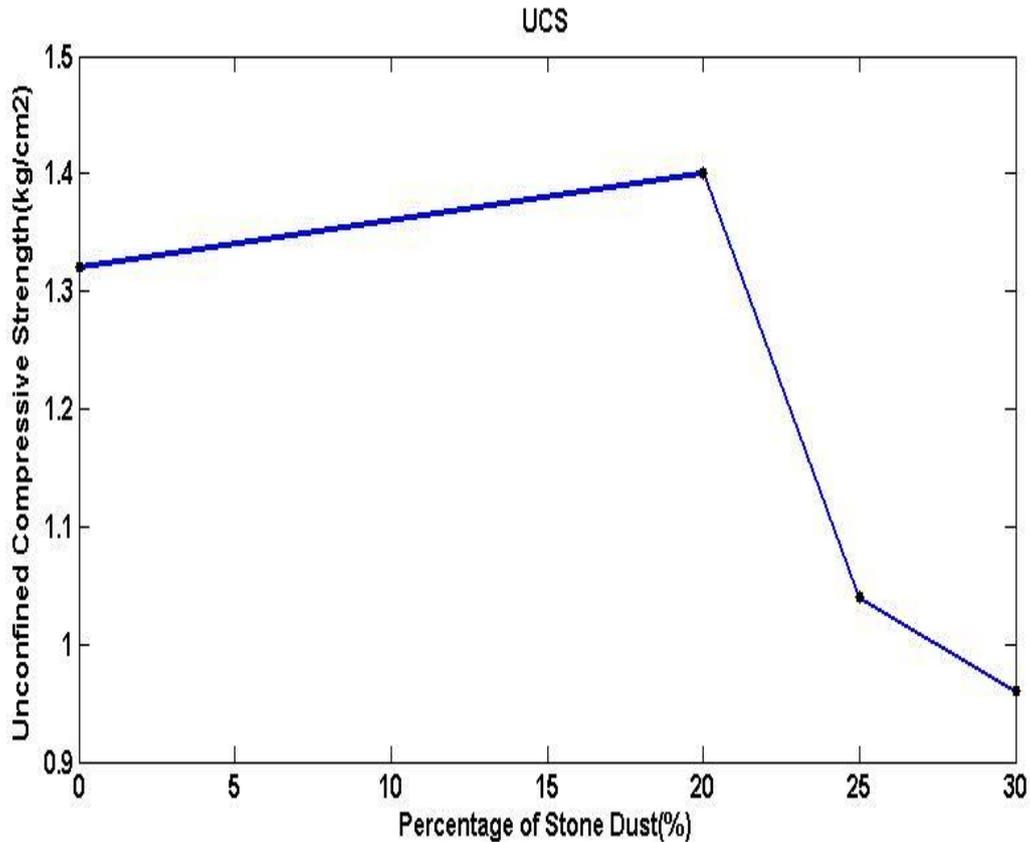
**Fig 22. Variation on Compressive Strength with % of stone dust**
