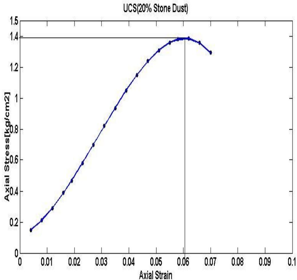
**Fig 11. Compressive Strength of soil with 20% stone dust**
