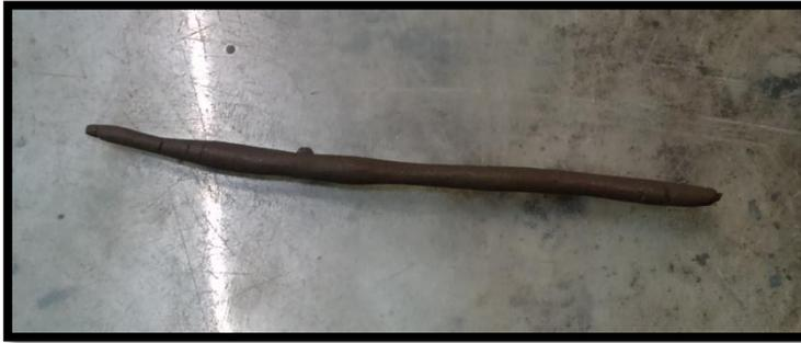
**Rolling of soil into threads of 3mm diameter**
