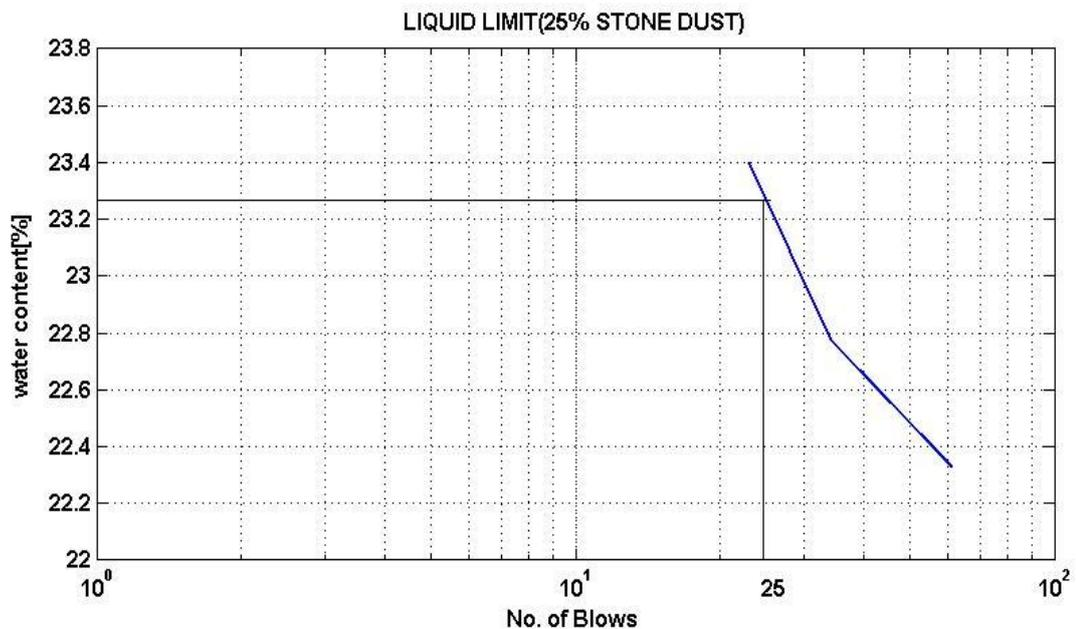
**Fig 17. Liquid Limit of soil with 25% stone dust**
