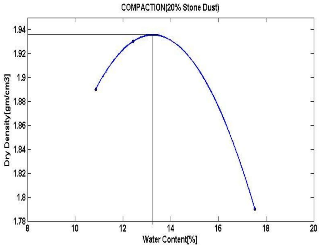
**Fig 7. Density- moisture content relationship of soil with 20%stone dust**
