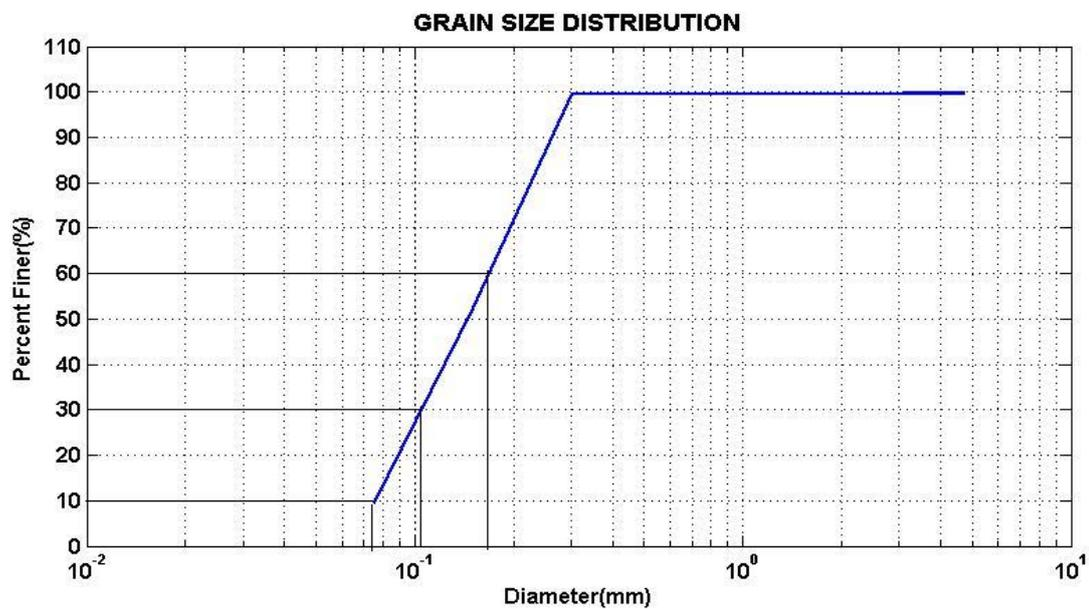
**Fig 6. Grain Size Analysis of Stone dust**
