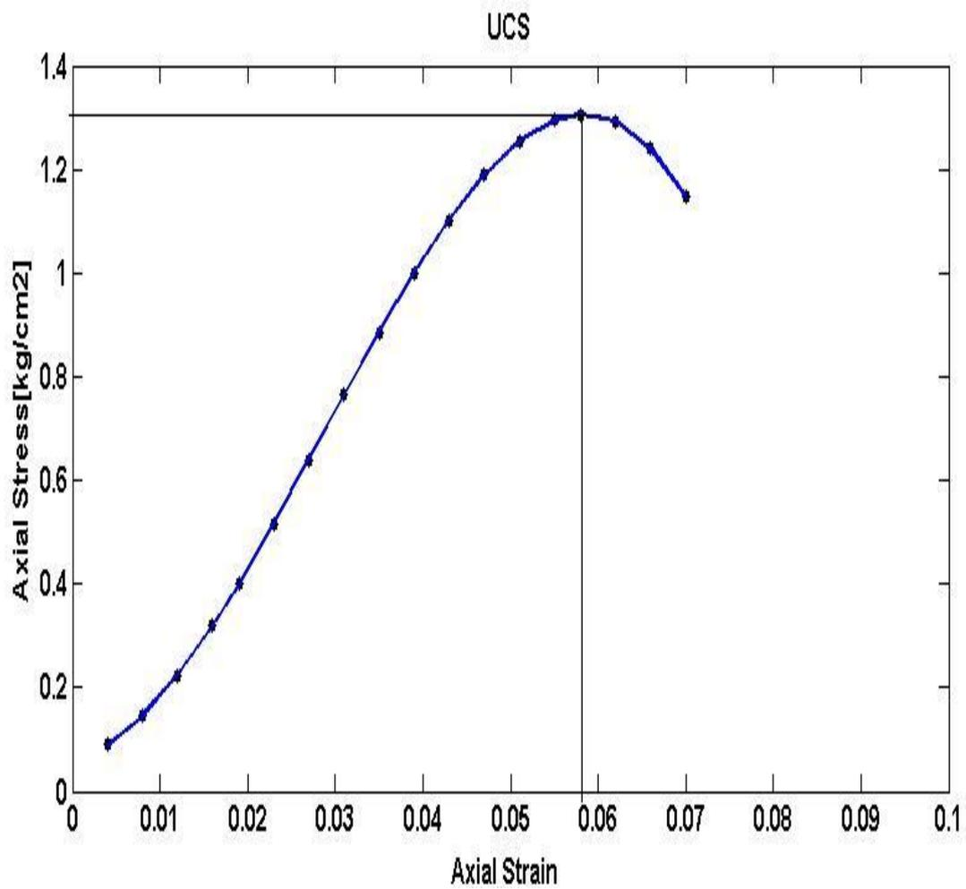
**Fig 4. Compressive strength of soil**
