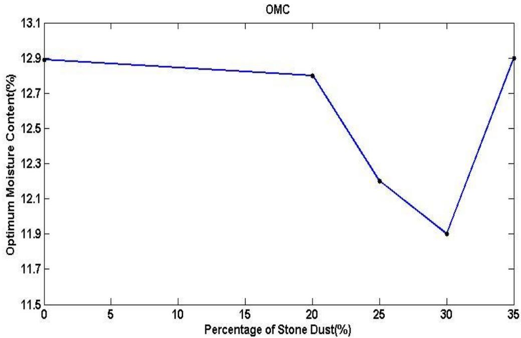
**Fig 21. Variation of optimum moisture content with % of stone dust**
