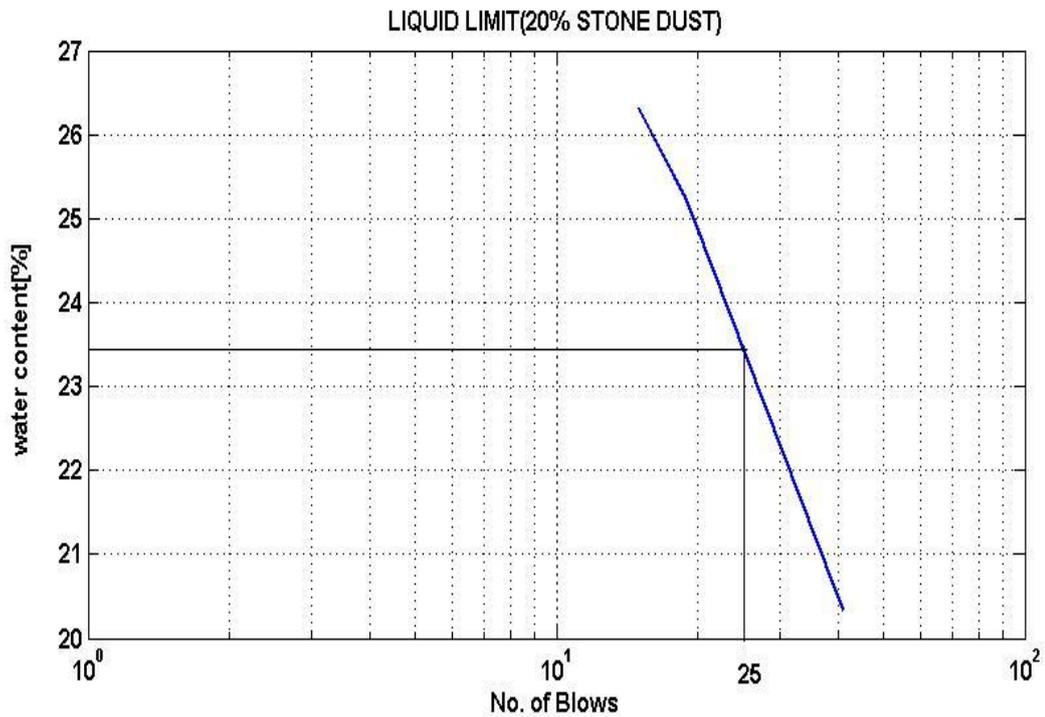
**Fig 16. Liquid Limit of soil with 20% stone dust**
