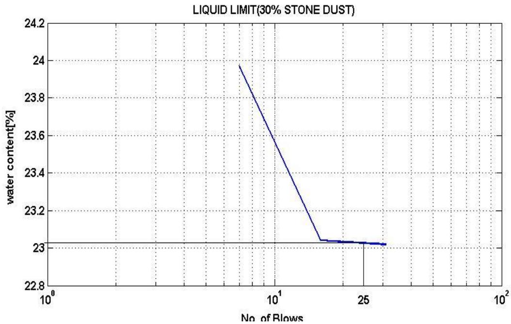
**Fig 18. Liquid Limit of soil with 30% stone dust**
