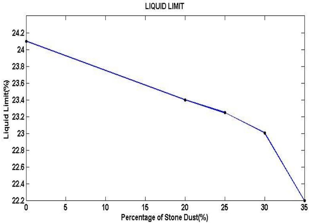
Fig 25. Variation on Liquid Limit with % of stone dust
