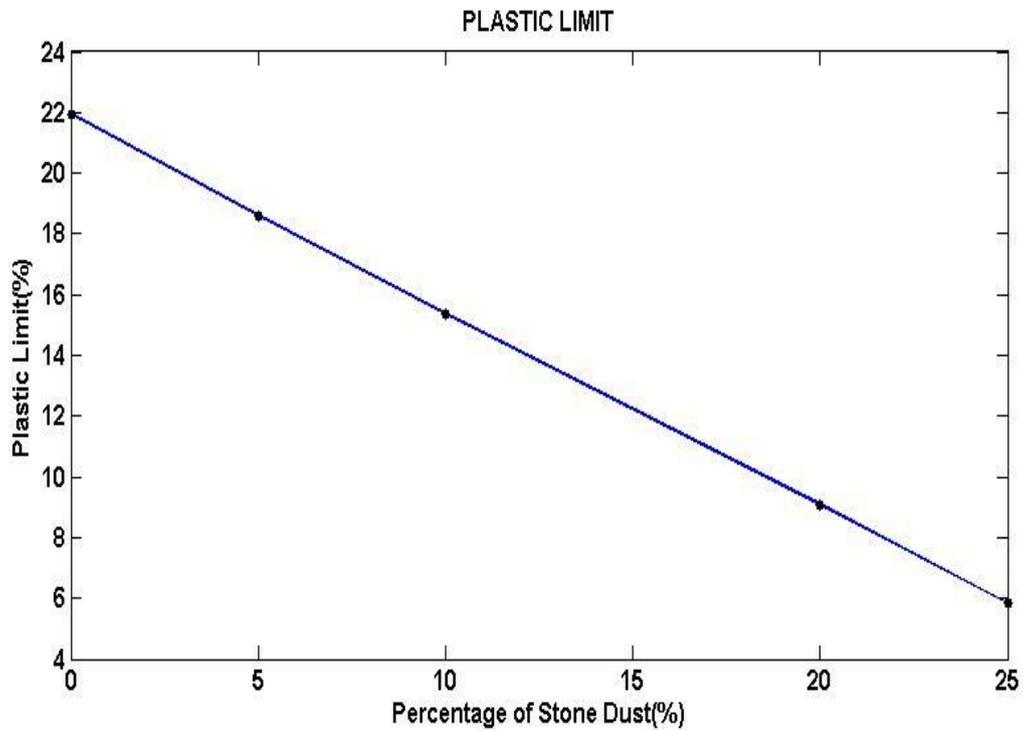
Fig 26. Variation on Plastic Limit with % of stone dust
