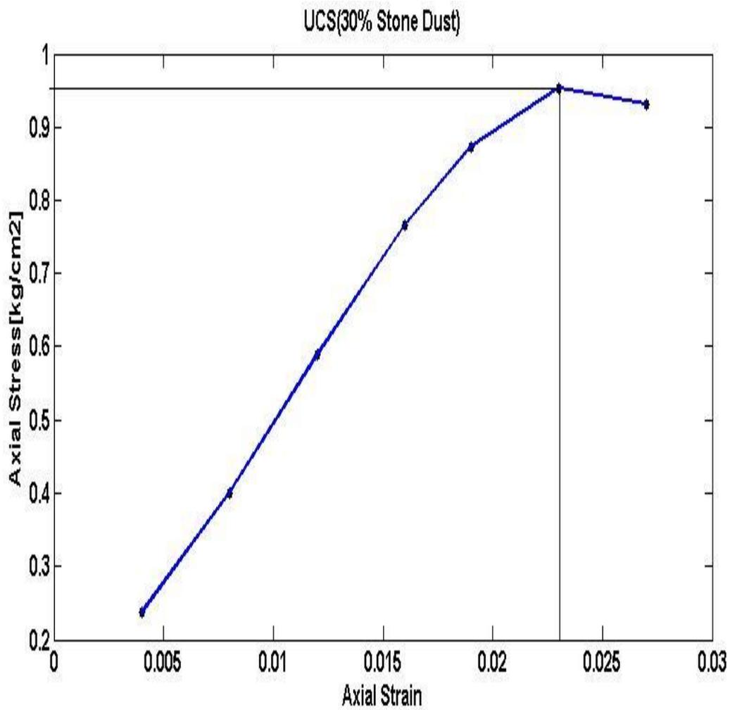
**Fig 13. Compressive Strength of soil with 30% stone dust**
