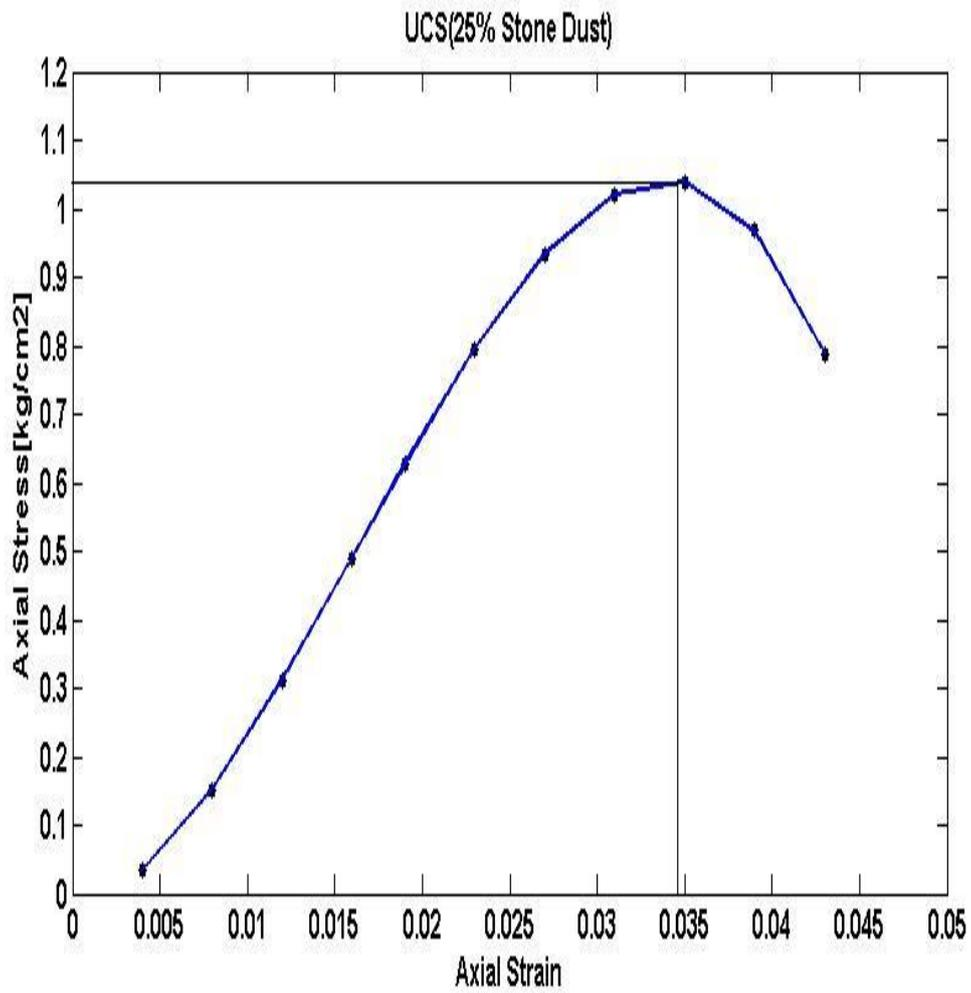
**Fig 12. Compressive Strength of soil with 25% stone dust**
