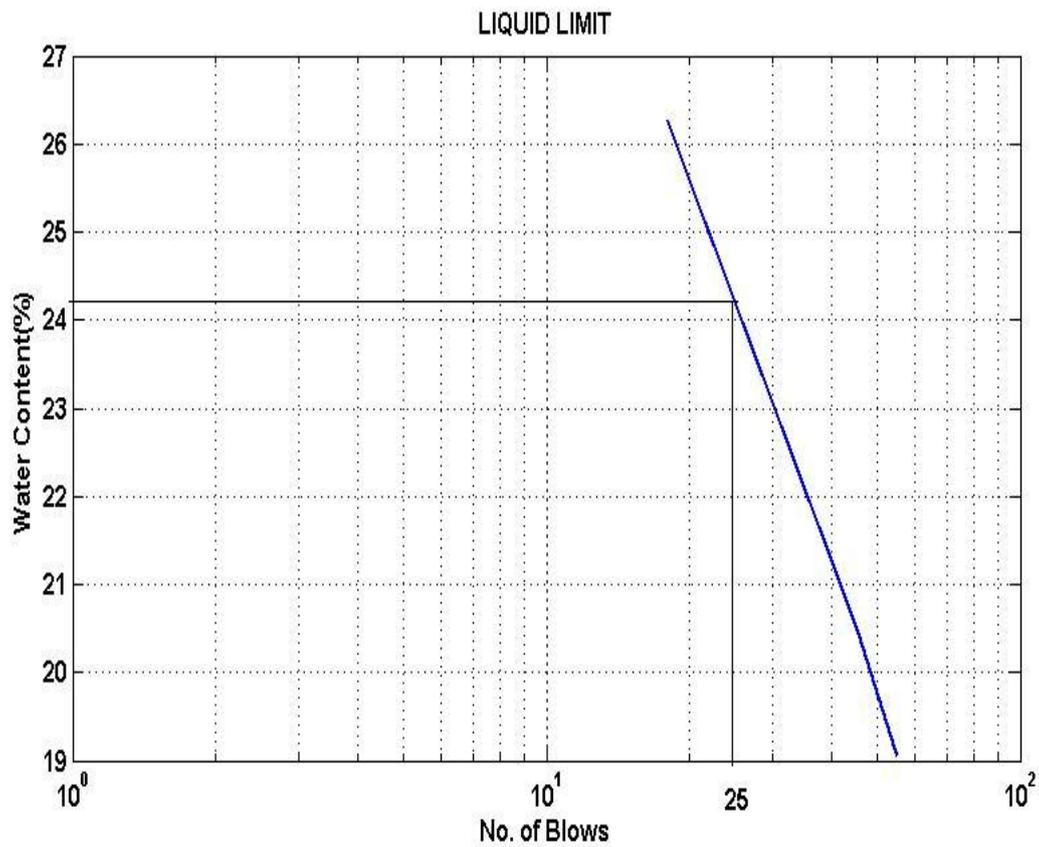
**Fig 2. Liquid Limit of soil**
