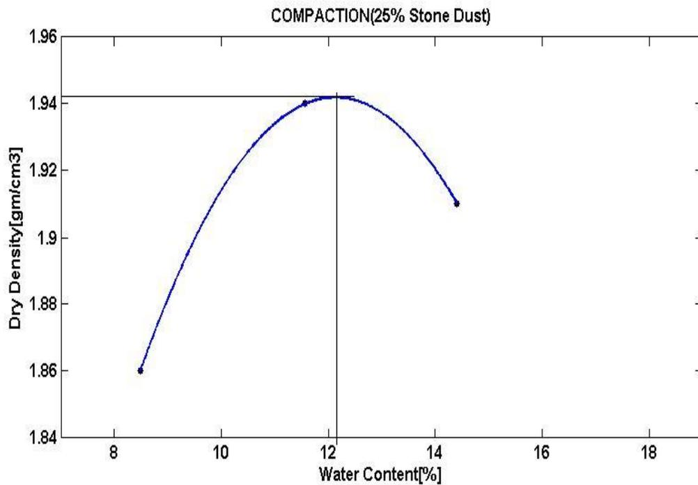
**Fig 8. Density- moisture content relationship of soil with 25% stone dust**
