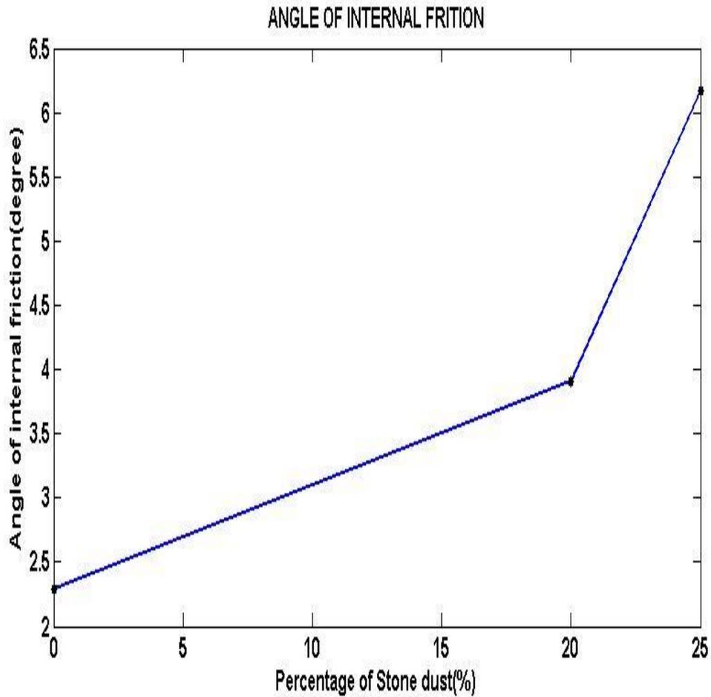
**Fig 24. Variation on Angle of Internal Friction with % of stone dust**
