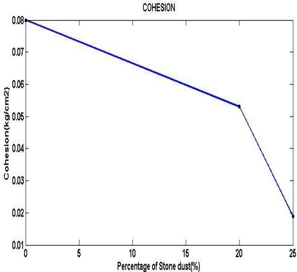
**Fig 23. Variation on cohesion with % of stone dust**
