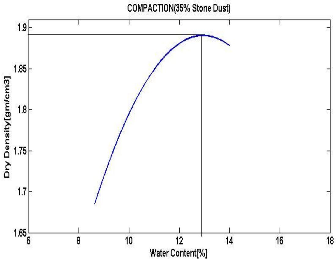
**Fig 10. Density- moisture content relationship of soil with 35% stone dust**
