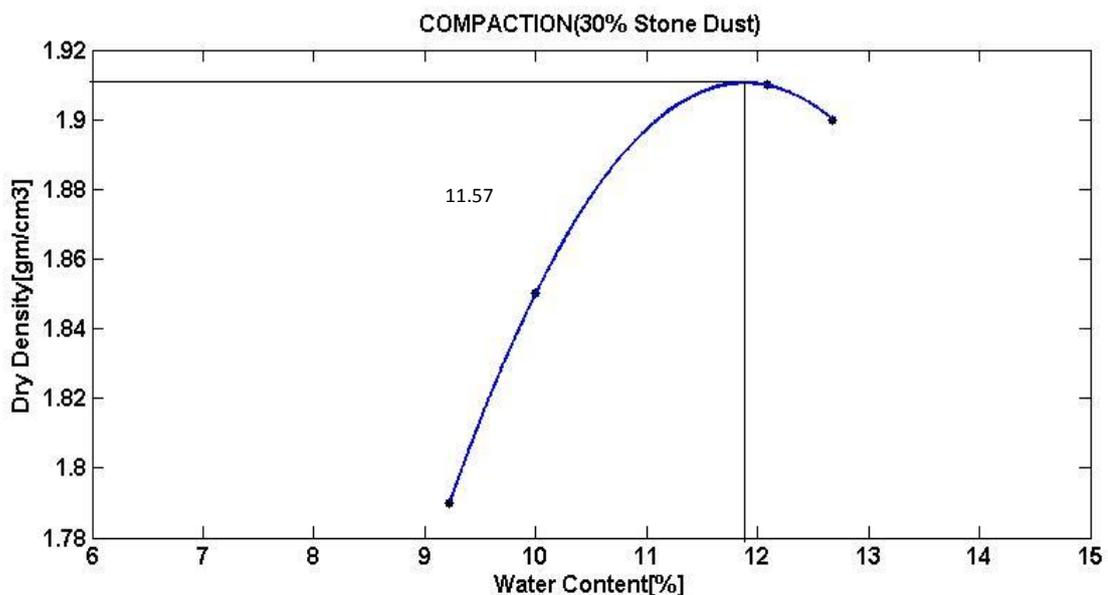
**Fig 9. Density- moisture content relationship of soil with 30% stone dust**
