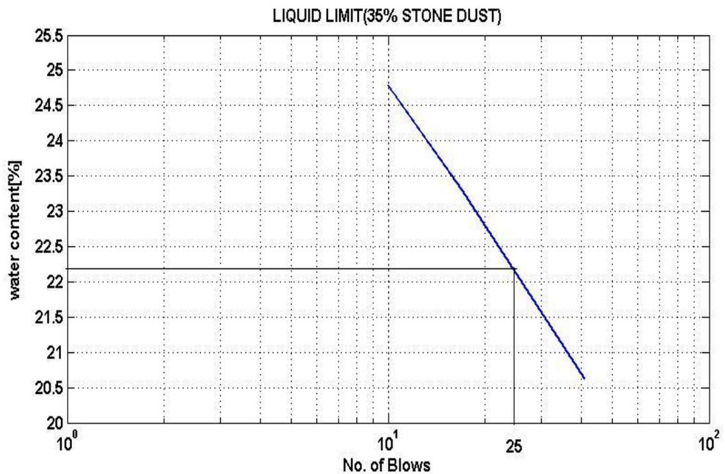
**Fig 19. Liquid Limit of soil with 35% stone dust**
