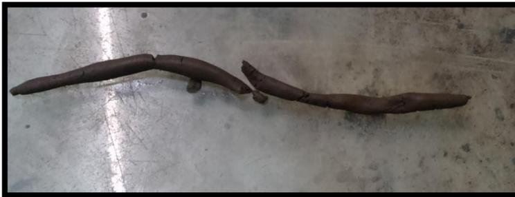
**Thread at diameter of 3mm just starts crumbling**
