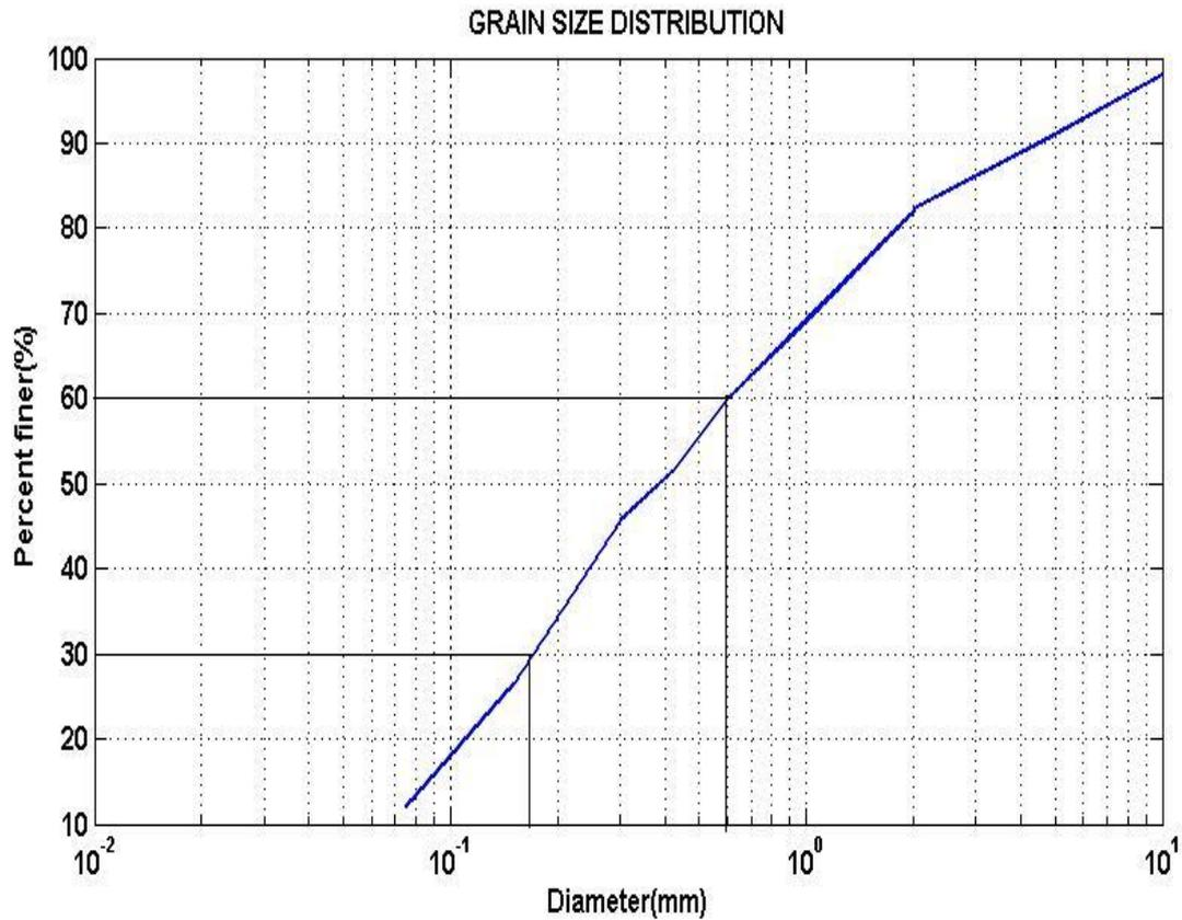
**Fig 1. Grain Size Analysis of soil**
