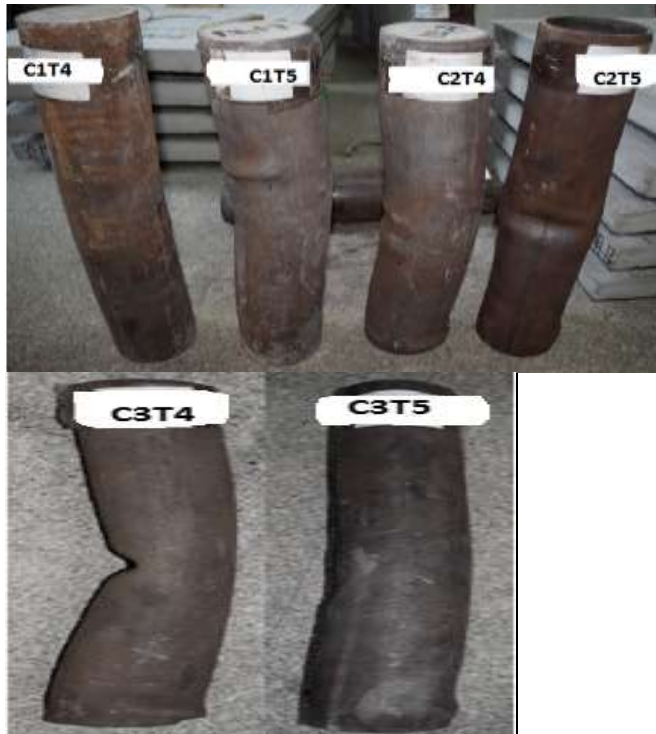
Figure 6 Failure Mode of CFST Circular Columns Under Axial Loading
