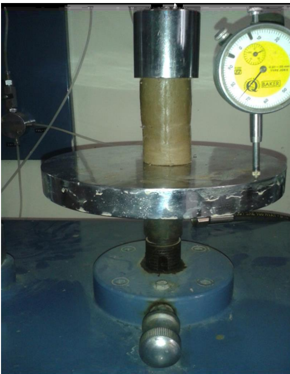
Figure 4: Unconfined compressive strength test
