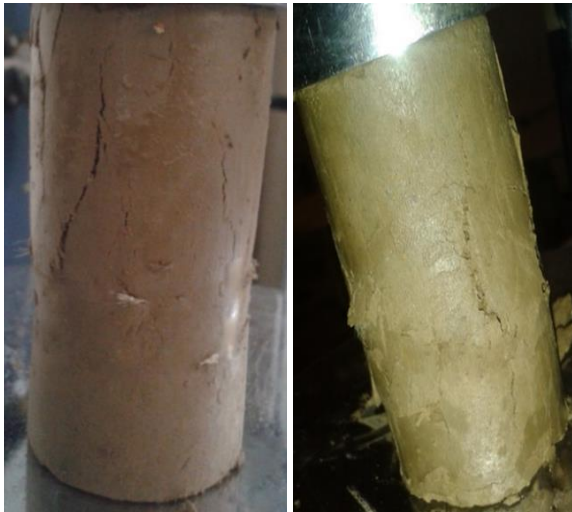
Figure 10: Failure with Non-Woven Geotextile when kept in between the failure plane
