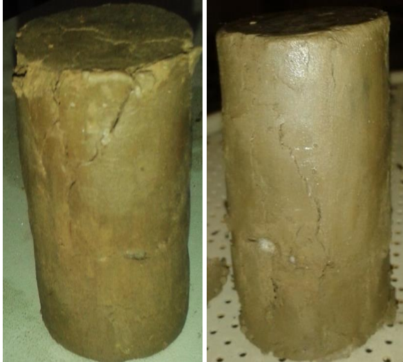
Figure 9: Failure with Woven Geotextile when kept in between the failure plane
