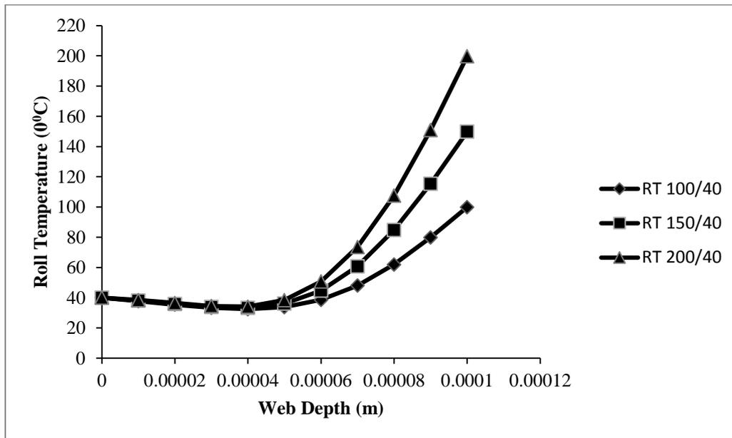
Fig.1. Impact of temperature of roll on fabric temperature at different depths
