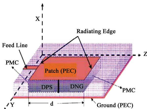
**Figure 1.** 3D view of DPS-DNG substrate for a rectangular microstrip patch antenna
