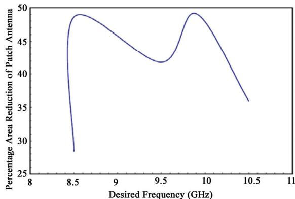
**Figure 4. Percentage reduction in the size of radiating patch for a desired frequency with CSRR as compared to without CSRR in the ground plane**
