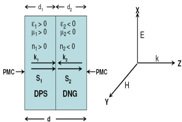
**Figure 2.** 1D cavity resonator made with DPS-DNG combination
