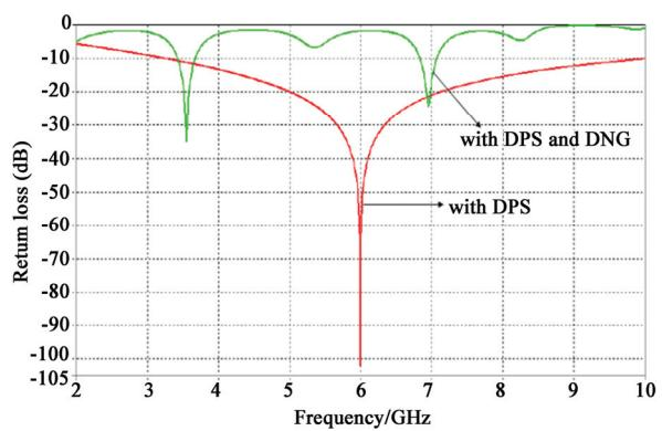
**Figure 3** Frequency downshifts in the slab made by DPS and DNG
