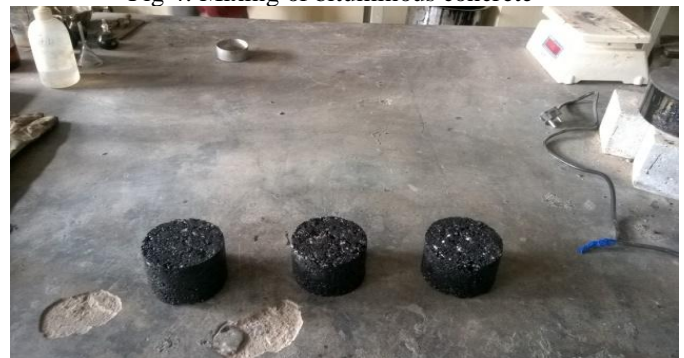
Fig 5: Bituminous samples with different Zycotherm concentration
