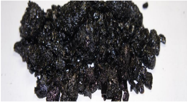
Fig 6: Aggregates after stripping test
