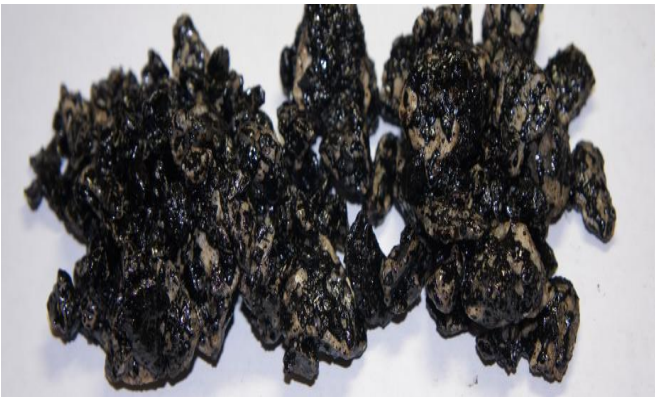
Fig 2: Aggregates coated with bitumen after the test
