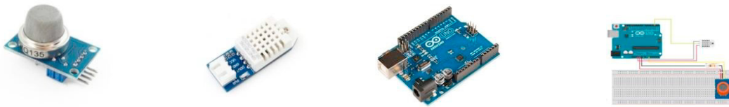
Fig.1. MQ-135 Gas Sensor [8] DHT-22 Humidity-Temperature Sensor [9] Arduino-Uno Microcontroller [10] Circuit Diagram
