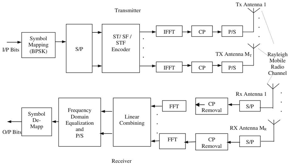
**Fig. 1** ST/ SF / STF coded  $M_T \times M_R$  MIMO-OFDM transceiver structure
