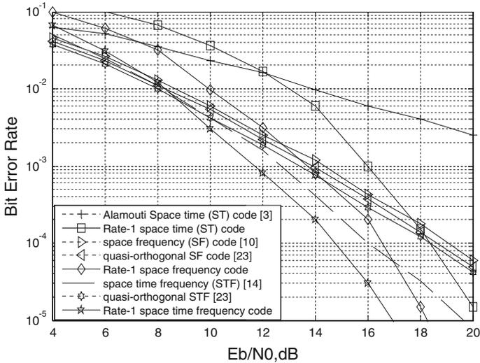
**Fig. 7** BER comparison of STFC and SFC with rate-1 for  $2 \times 1$  MIMO-OFDM system in quasi-static Rayleigh frequency flat channel
