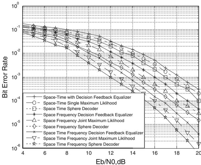
**Fig. 4** Comparison of BER for BPSK using  $2 \times 1$  MIMO-OFDM system in quasi-static Rayleigh frequency selective channel
