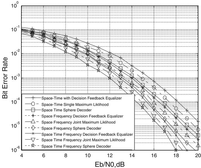
**Fig. 6** Comparison of BER for BPSK using  $2 \times 2$  MIMO-OFDM system in quasi-static Rayleigh frequency selective channel
