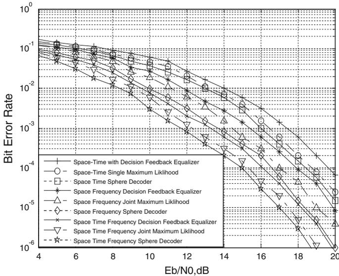
**Fig. 3** Comparison of BER for BPSK using  $2 \times 1$  MIMO-OFDM system in quasi-static Rayleigh frequency flat channel
