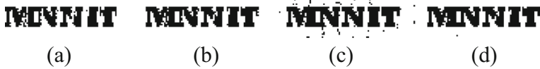
Fig. 5 Extracted Health Center's logo with pfa at (a) 10^{-2} (b) 10^{-3} (c) 10^{-6} (d) 10^{-8} at level 1
