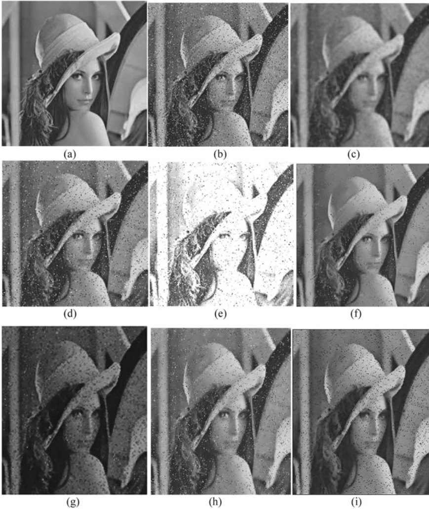
Fig. 3 a Original Lena image. b Noisy image (speckle noise = 10%). c Frost filtered image. d PM filtered image. e DPAD results. f OBNLM. g ADMSS. h Guided filter. i DMF
