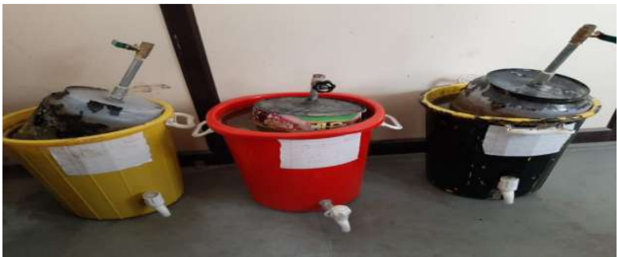
Figure 3.5: –Digesters D2,D4 and D6 placed at controlled temperature of 25 °C
