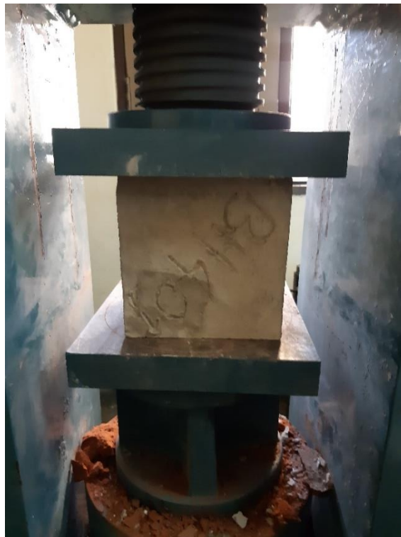
Figure 3.10: Testing of cube using compression testing machine
