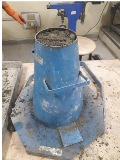
Figure 3.8 Determination of workability by slump cone test
