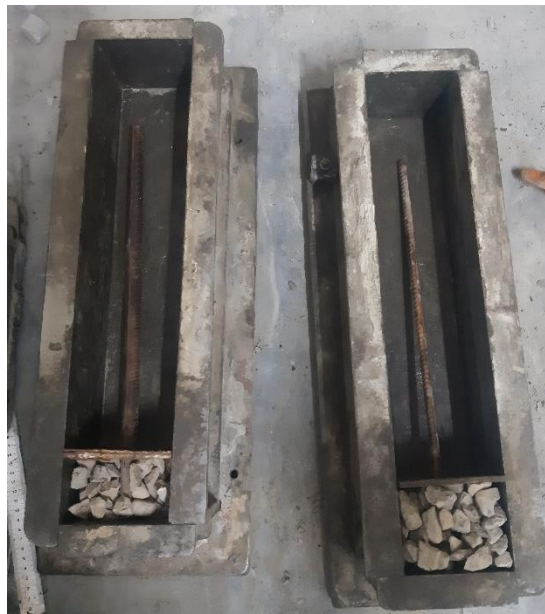
Figure 3.11 Concrete beam mould
