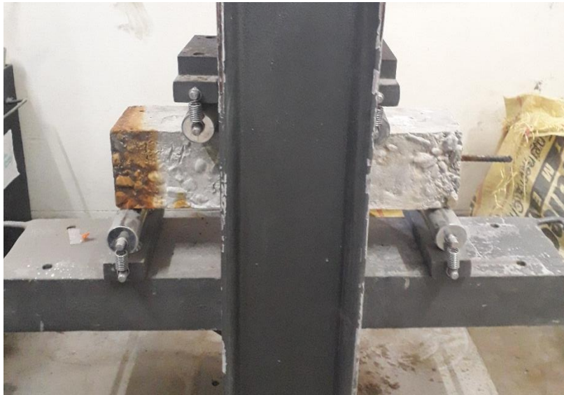
Figure 4.1: Testing for flexural strength
