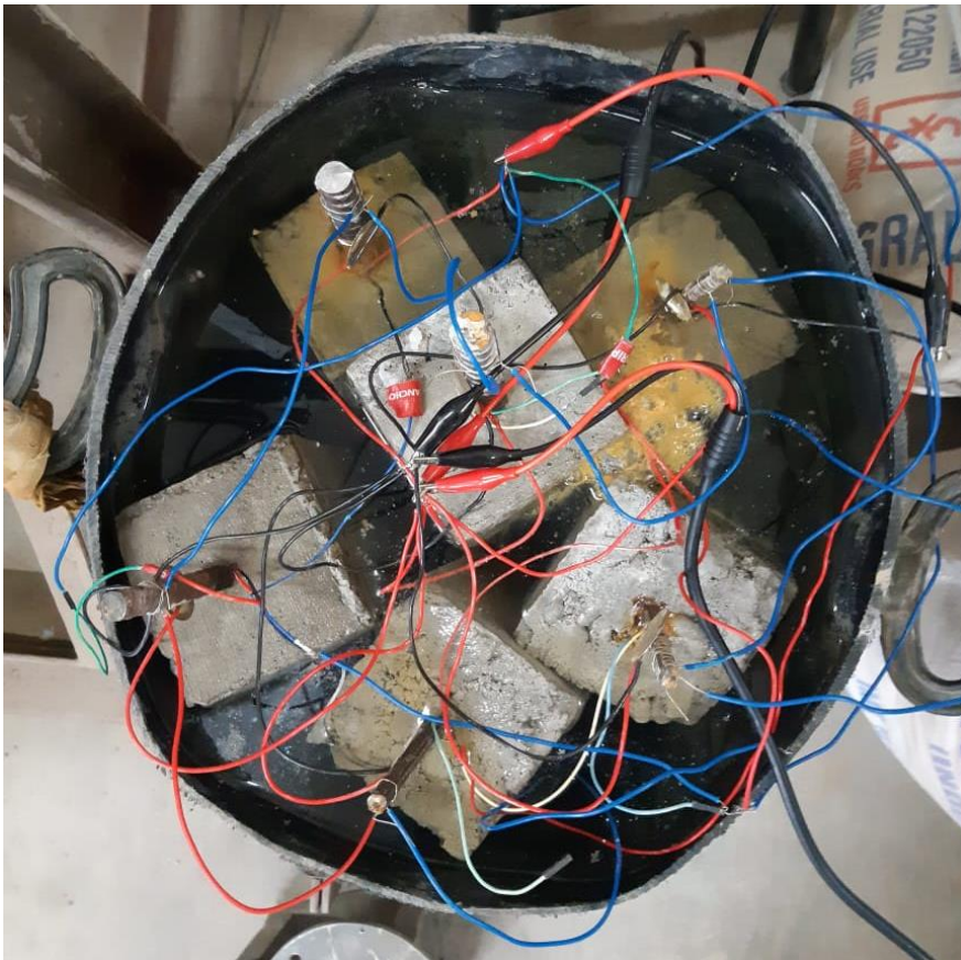
Figure 3.15: Experimental set up of impressed current methods
