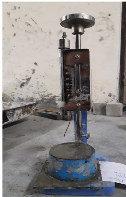
Figure 3.1 Determination of normal consistency of cement using Vicat apparatus
