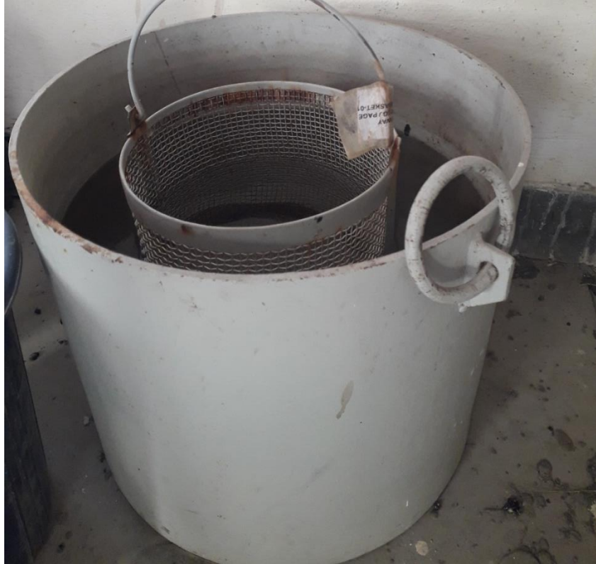
Figure 3.7 water absorption test by density bucket
