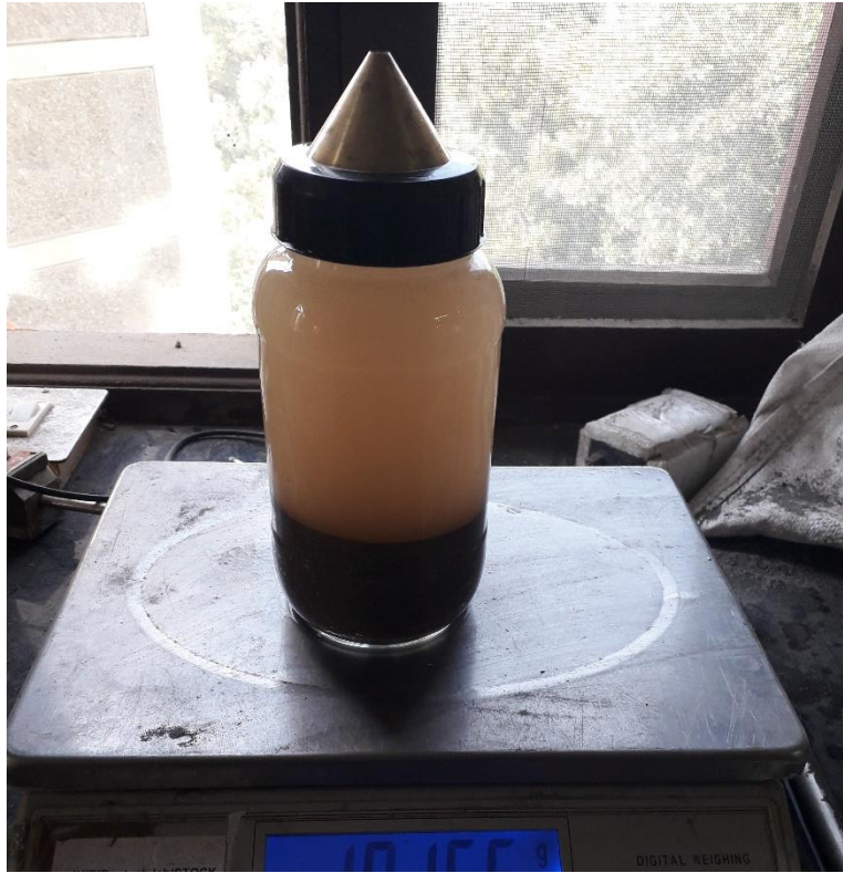
Figure 3.6 Determination of specific gravity of sand using pycnometer
