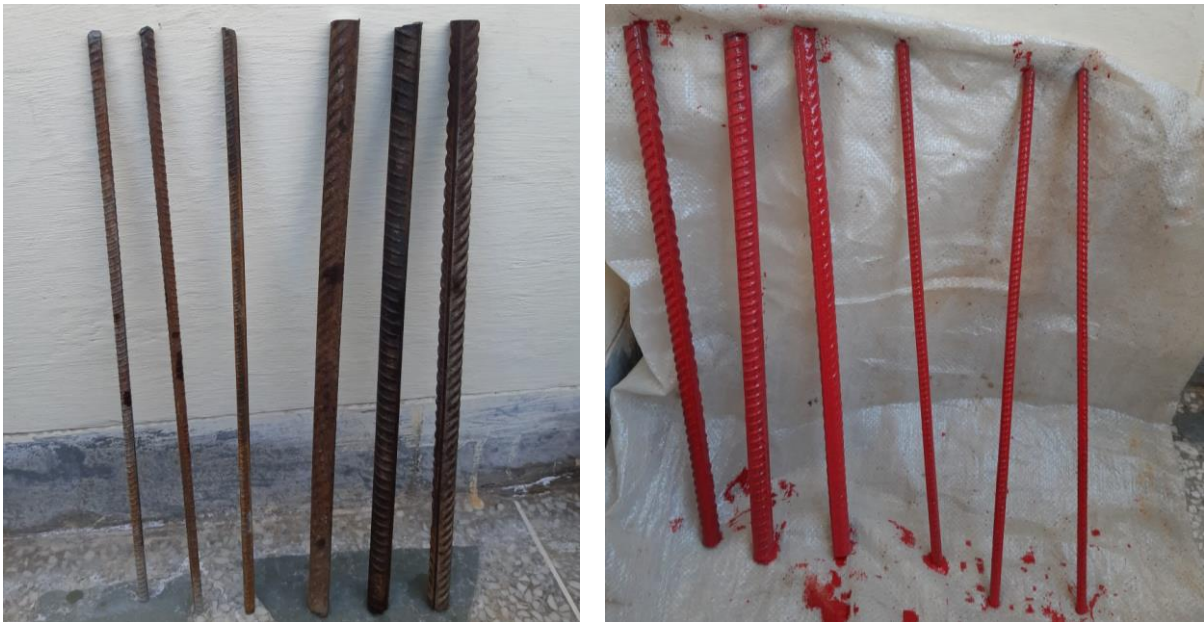
Figure 3.16: Rebar embedded in beam casted without and with inhibitor
