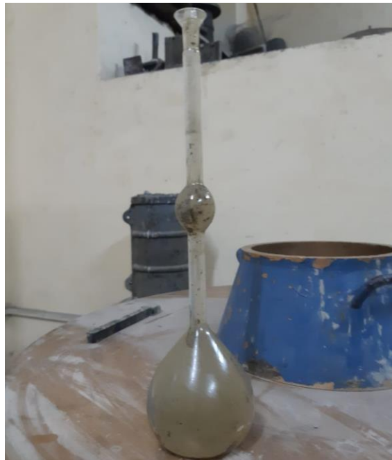
Figure 3.4 Determination of specific gravity of cement using Le Chatelier's flask
