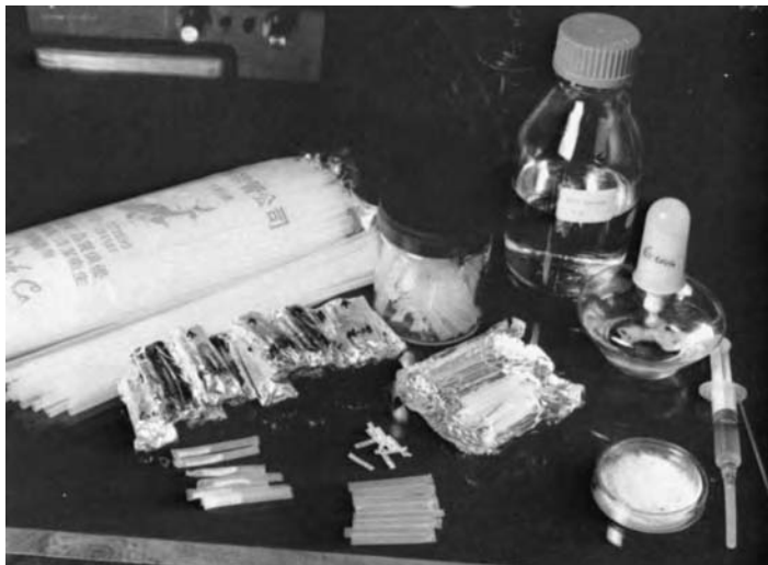
FIGURE 10.6 The short drinking straw, the small labels, and the prepared straw ampoules wrapped in small packages with aluminum foil and labeled on the outside by marker pen.
