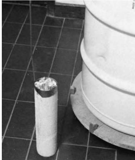
FIGURE 10.8 A canister of the BT37 with ampoule packages inside. Each canister can accommodate as many as 28 to 30 packages.
