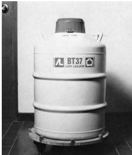
FIGURE 10.9 The BT37 liquid nitrogen tank of the L' Air Liquide Cryogenic Equipment division.
