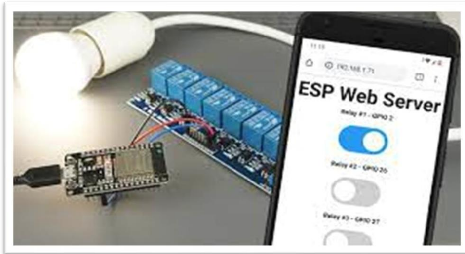
Figure 2.7: Web portal controlling the bulb with ESP32 board
