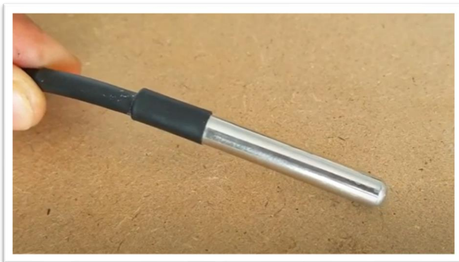
Figure 3.2: DS18B20 Temperature sensor (waterproof)
