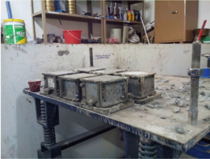
Fig. 1 Cubes being casted and on vibrating table
