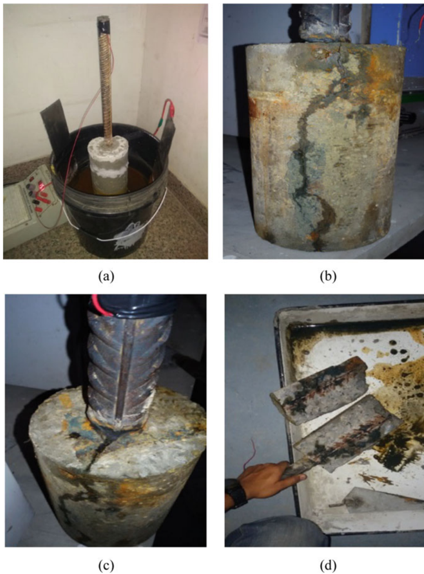
Fig. 3 (a) Laboratory ICT setup, (b) crack propagation along the surface, (c) crack initiation from free top surface along the steel bar, (d) steel bar removal after breaking of RC specimen
