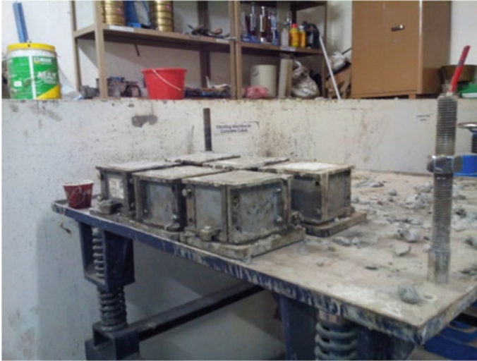
Fig. 1 Cubes being casted and on vibrating table
