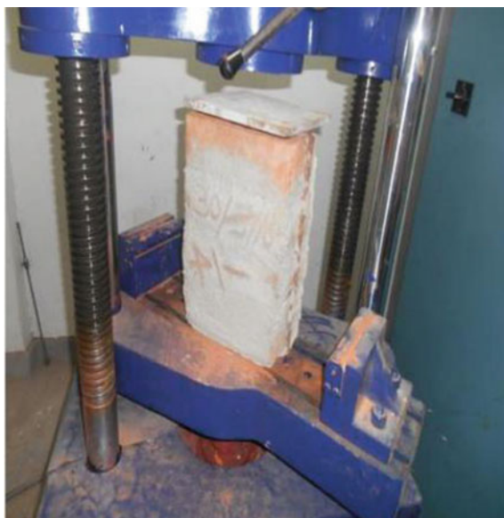
Fig. 10 Confined masonry failure
