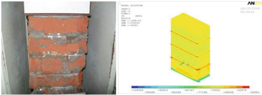
Fig. 3 X-component of stress on UTM and ANSYS
