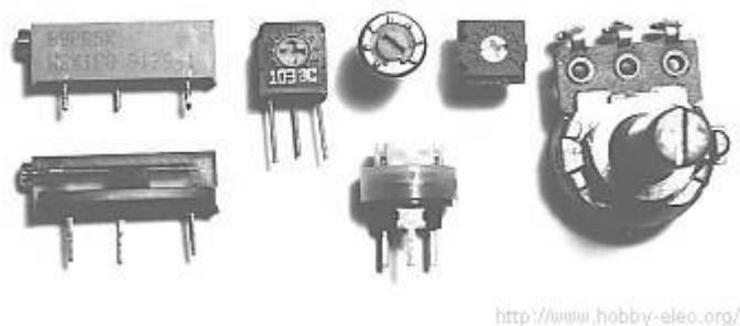
Fig 17. VARIABLE RESISTORS
