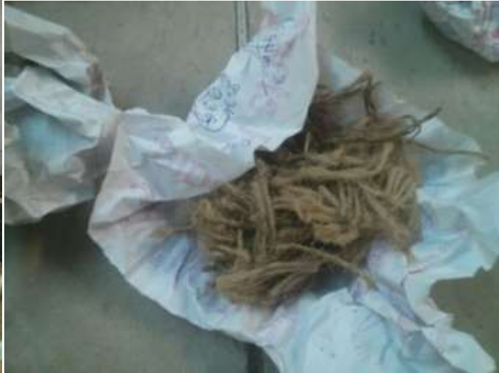
Fig.4 Jute Strips after cutting
