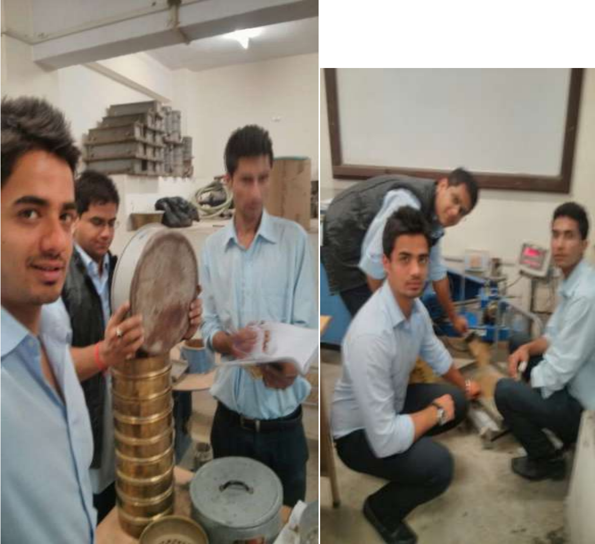
Fig. 7 PERFORMING SEIVE ANALYSIS FOR GSD
