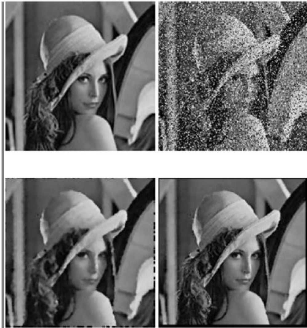
Fig. 9: Results of filtering with a 5X5 median and conditional median filter. From left to right, first row : original Image, noisy image. second row : standard median filter, Adaptive median filter.
