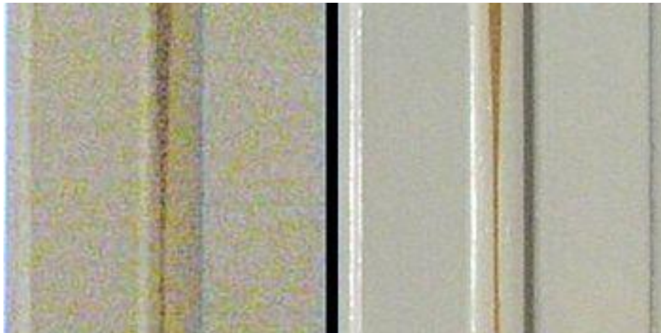
Fig. 6: Image on the left has exposure time of >10 seconds in low light. The image on the right has adequate lighting and 0.1 second exposure.
