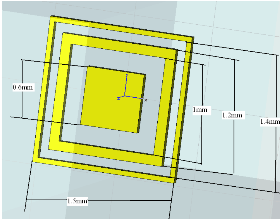
Figure: 3.7 Dimensions of double square loop with a patch type element
