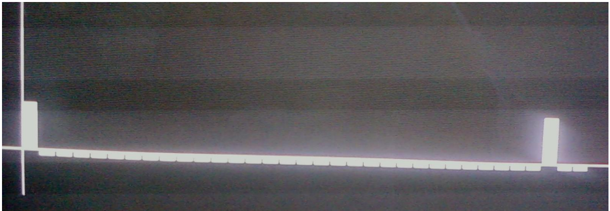
Snapshot5:- This snapshot shows Periodic Autocorrelation of 31 lengths PN-Sequence.
