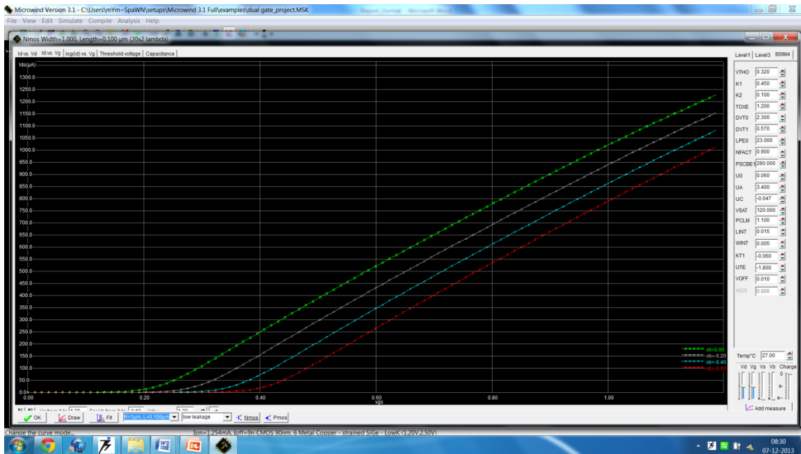
Figure 36 – Transfer Characteristics of Dual Gate MOSFET
