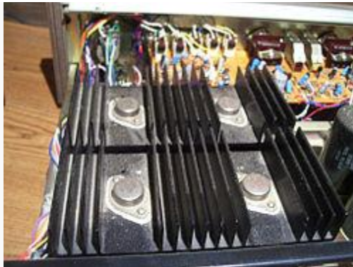
Figure 47 - Large Heat Sinks To Cool Power Transistors In Atrm-800 Audio Amplifier
