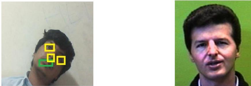
Figure 10: Test Image (a) and train database image (b) . Under different Lighting conditions and varying distance faical recogniton positive using PCA analysis. If Minimum Euclid<0.8e008 and 0.35e008 facial recognition is positive as seen in table 7 where test image matches to training Image 2 as the minimum Euclidian distance is 0 in all the test cases
