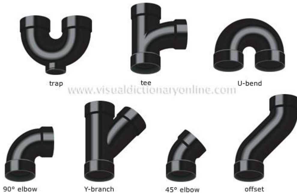
Fig.2.10.1: Fittings Used for Connections
