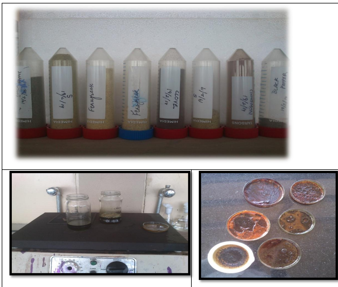
Fig4: Preparation of extracts (a) powdered spices, (b) Heating on hot plate to evaporate methanol (c) Residue of spices
