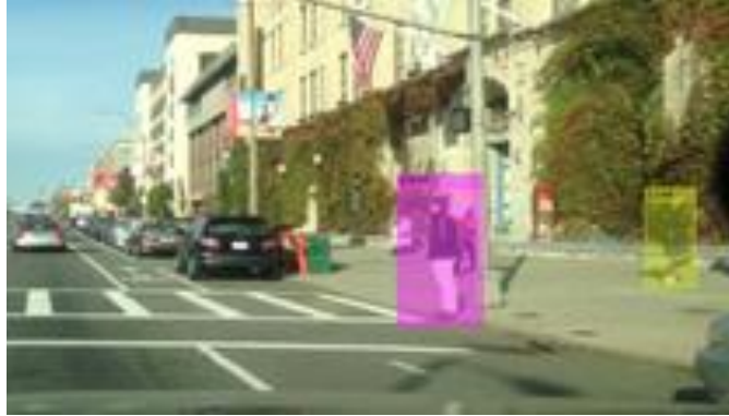
FIGURE 4.18: People detector Detecting people using pretrained support vector machine(SVM) with histogram of oriented gradient (HOG) features
