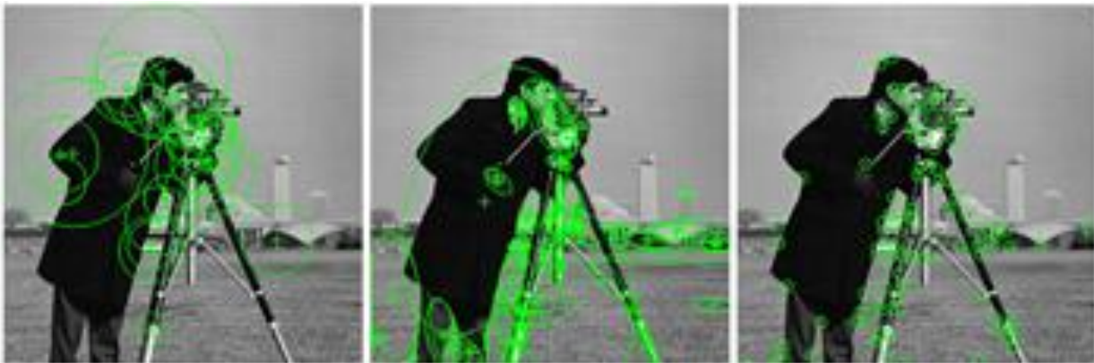
FIGURE 4.14: SURF (left), MSER (center), and corner detection (right) with Computer Vision System Toolbox . Using the same image, the three different feature types are detected and results are plotted over the original image.
