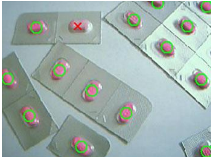
FIGURE 4.13: Image of blister packs acquired by Image Acquisition Toolbox. Image Processing Toolbox analyzes the data and marks broken pills.
