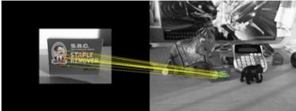
FIGURE 4.23: Reference image of object (left), input image (right); the yellow lines indicate the corresponding matched features between the two images.
