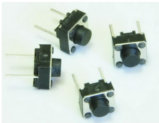
Figure 12: Push button switches [16]
