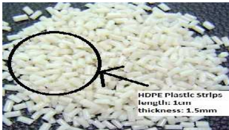
Fig.3: view of HDPE strips
