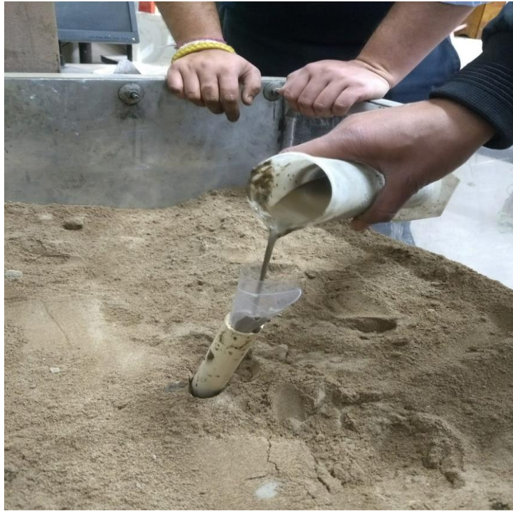
Fig. 3.18 Pouring Grout in Installed Pile
