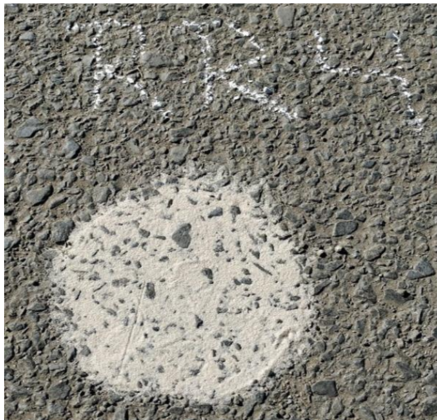
Fig.4.14: Sand Patch Test on RR-4
