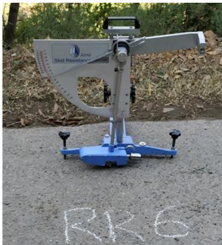
Fig. 4.13: Skid Resistance Testing at RR-6
