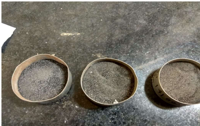
Fig 3.3 Untanned leather ash after heating at 200°C in incinerator
