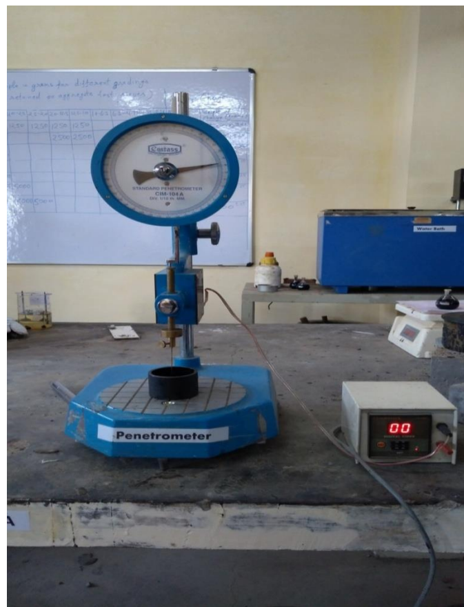
Fig 3.10: Penetrometer showing the penetration value.
