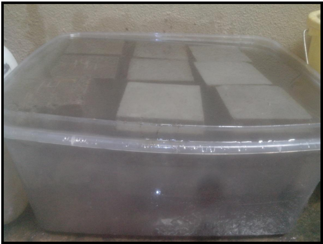
Figure 3.8 Cubes put for durability study (Sulphate attack)
