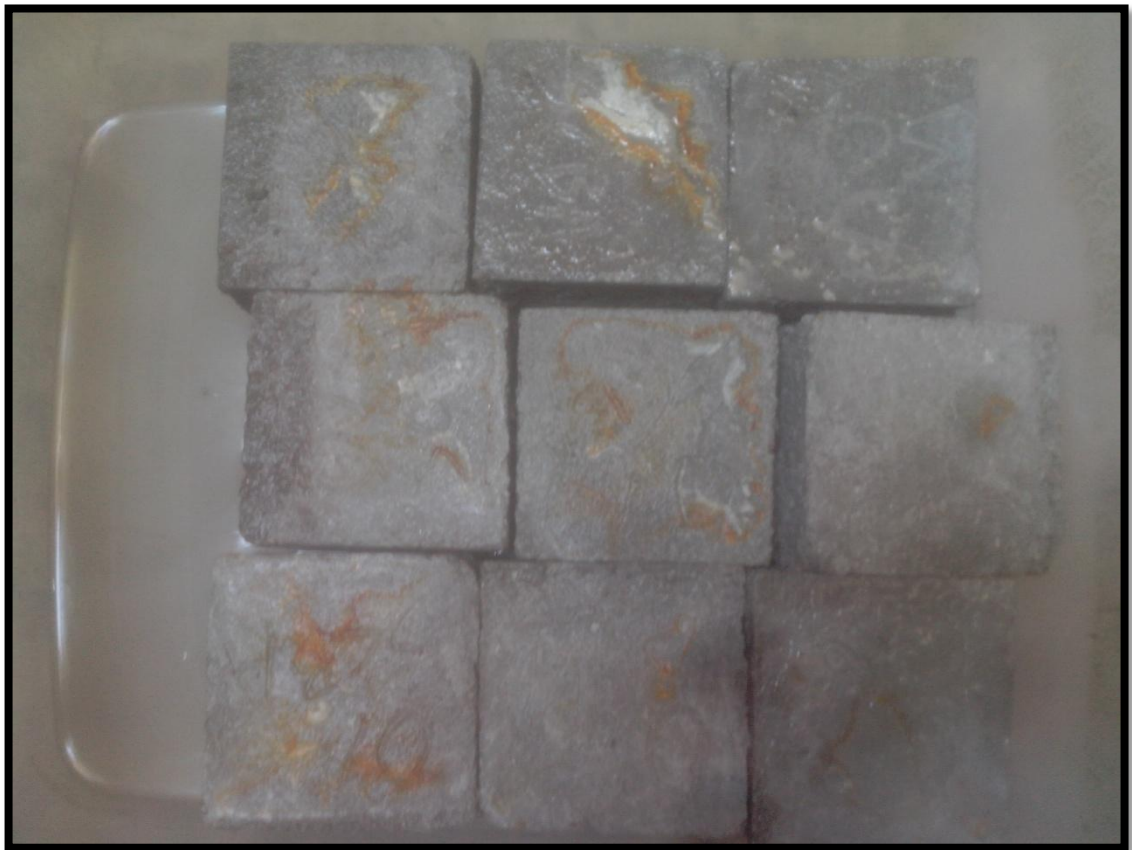
Figure 3.10 Condition of cubes after 21 days exposure to 5% H_2SO_4 solution
