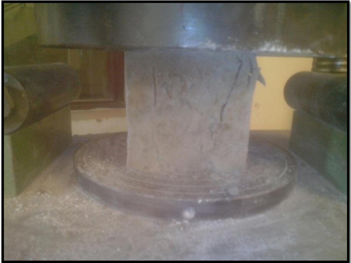
Figure 4.4 Cracks at failure in Compression testing of Cube (100mmx100mmx100mm)
