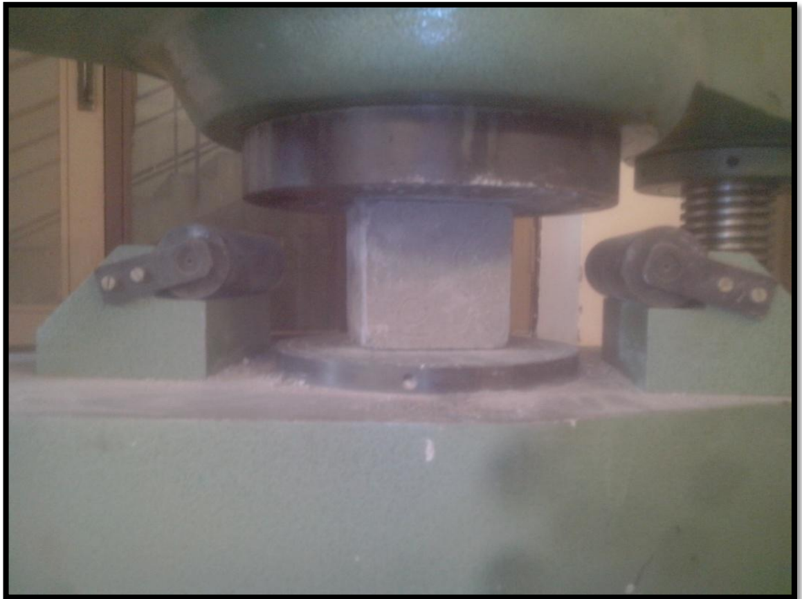
Figure 4.3 Compression testing of casted Cube (100mmx100mmx100mm)
