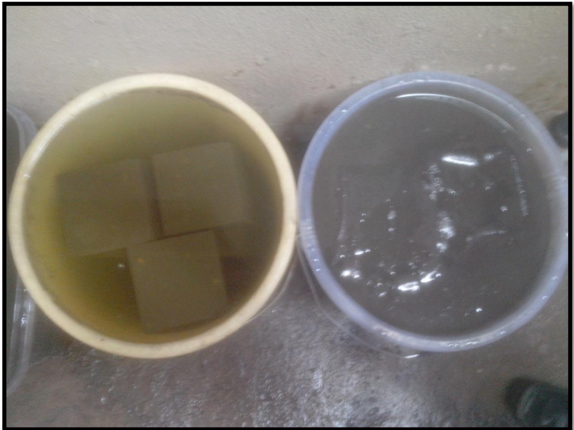
Figure 3.9 Cubes exposed to Hydrochloric Acid (5% Solution)
