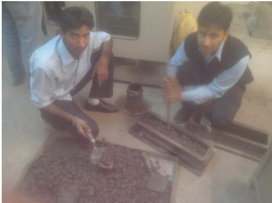
Figure 3.6 Casting the beam from mould (50x10x10 cm)
