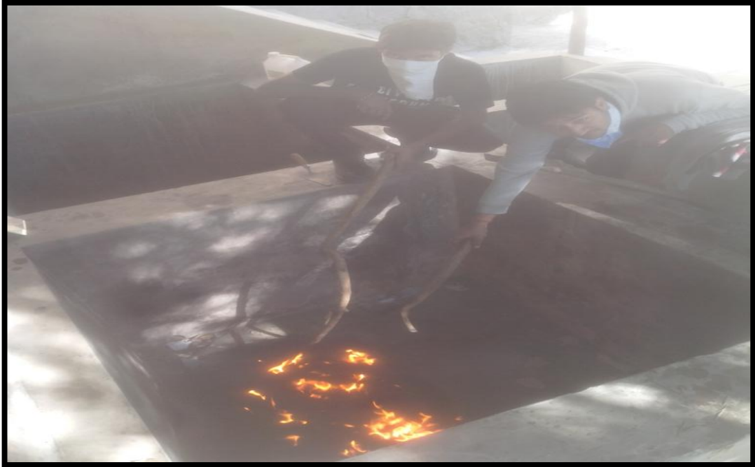
Figure 3.1 Open Field Incineration of Sugarcane Bagasse Ash procured from sugar mill
