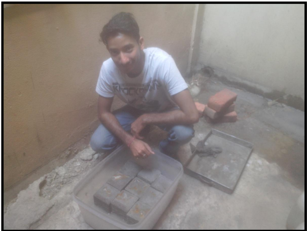
Figure 3.12 Student Vaibhav Gupta displaying Cubes exposed to Sulphate attack
