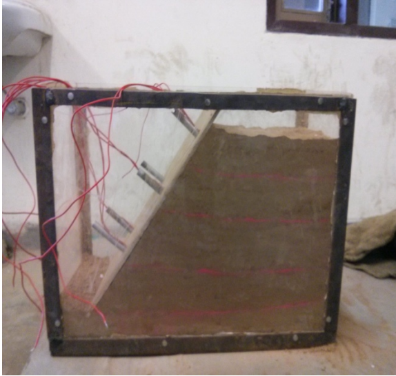
Fig 4.7 45° reinforced slope before failure.
