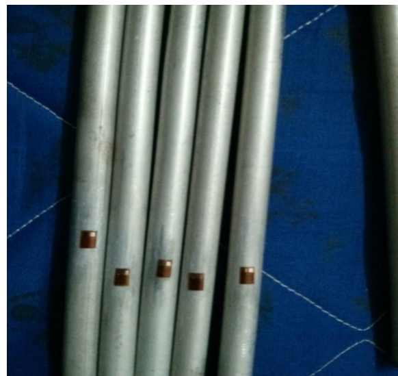
Fig 3.17 Strain gages glued to nails
