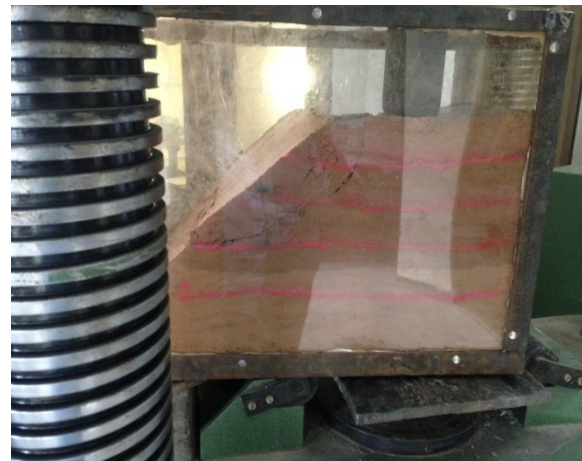
Fig 4.4 45° slope after failure
