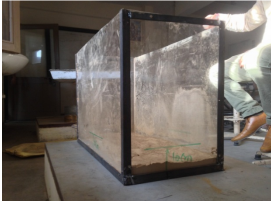
Fig.3.5 Base layer being laid in box.
