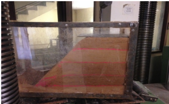
Fig 4.9 60° reinforced slope before failure.
