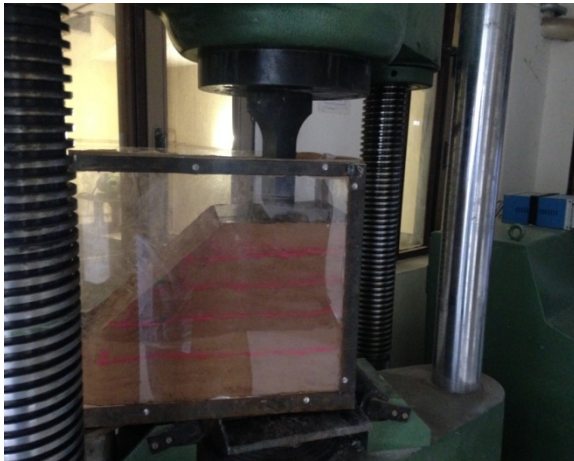
Fig 4.3 45° slope before failure
