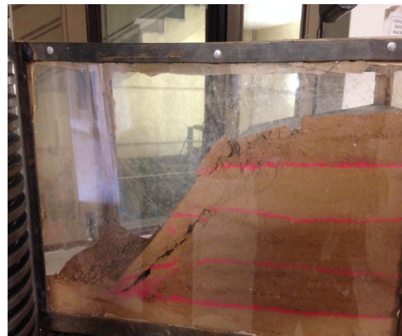
Fig 4.6 60° slope after failure
