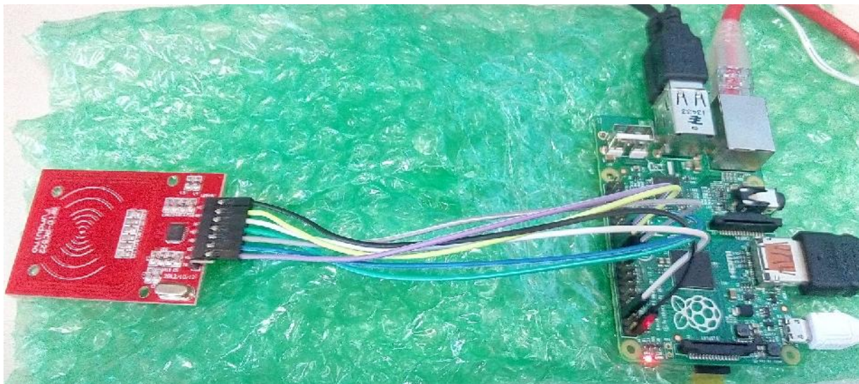
Figure 20: Raspberry Pi interfaced with MFRC522
