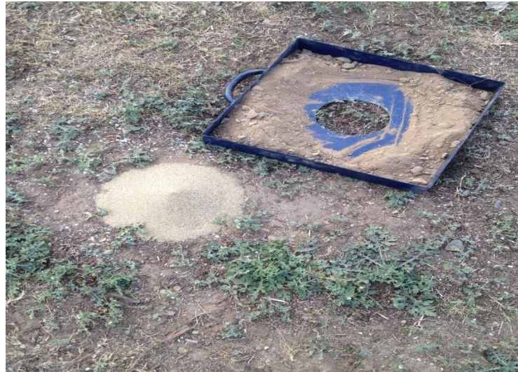
Fig. 3.6.2 Sand Replacement Method
