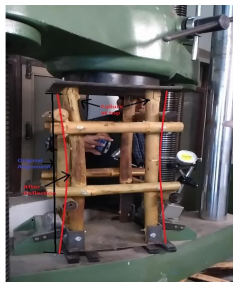
Fig. 20. Failure after load
