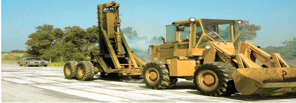
Figure 4.1. Trailer-mounted diesel hammer, one of the most common types of impact breakers
