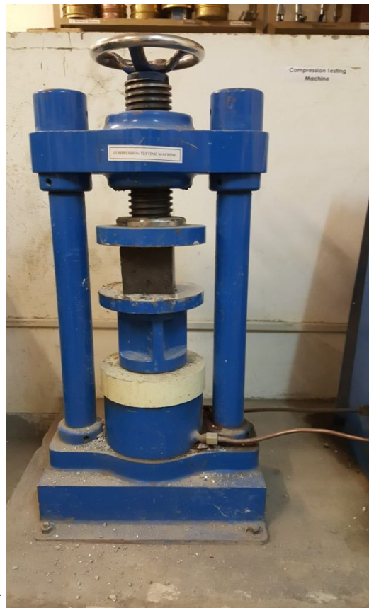
Fig 7.2 - Compressive Testing of Cube
