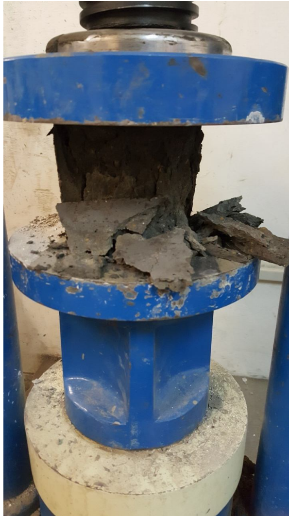
Fig 7.3 – Failed Cube after compression
