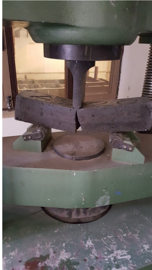
Fig 7.6 – Failed Beam Specimen
