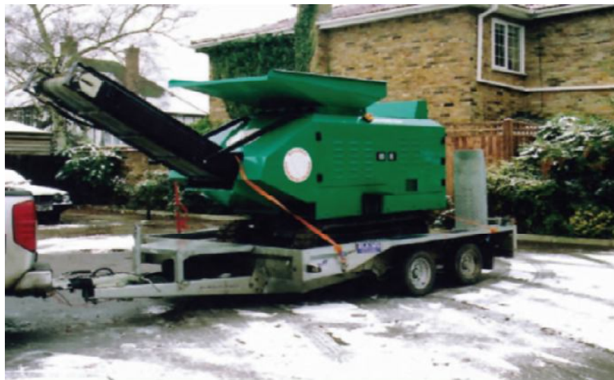
Figure 4.4 Aggregate Crushing Plant
