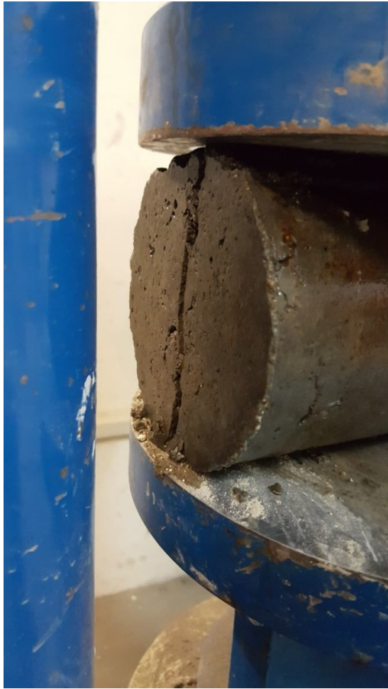
Fig. 7.5 – Failed Cylinder Specimen
