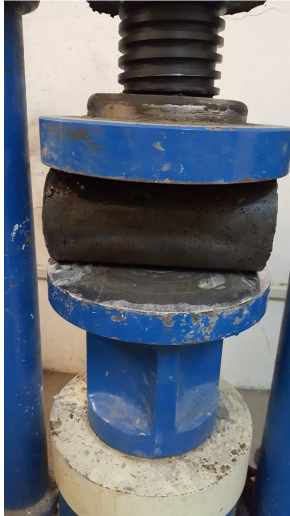
Fig. 7.4 – Cylinder in Split Tensile Test
