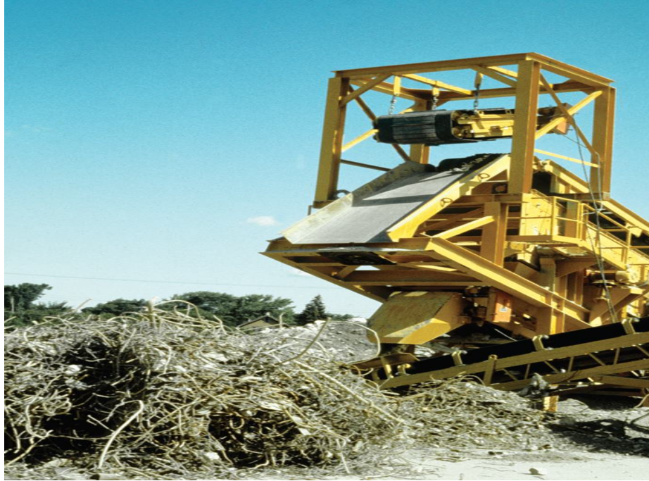
Figure 4.3 Conveyor belts with electromagnets
