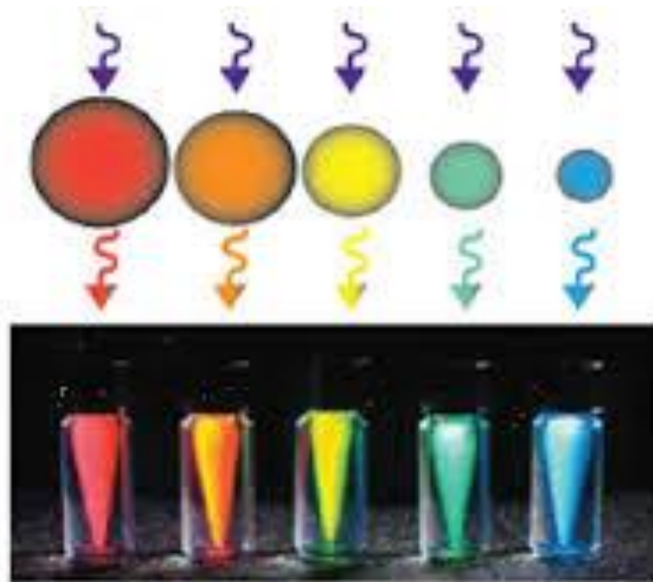
Fig. 1: The wavelength of light emitted by quantum dots is tunable by changing the particle size. In this image, all of the quantum dot samples are excited by the same wavelength, but emit different visible wavelengths depending on particle size. (Joshua James Angell 2011)
