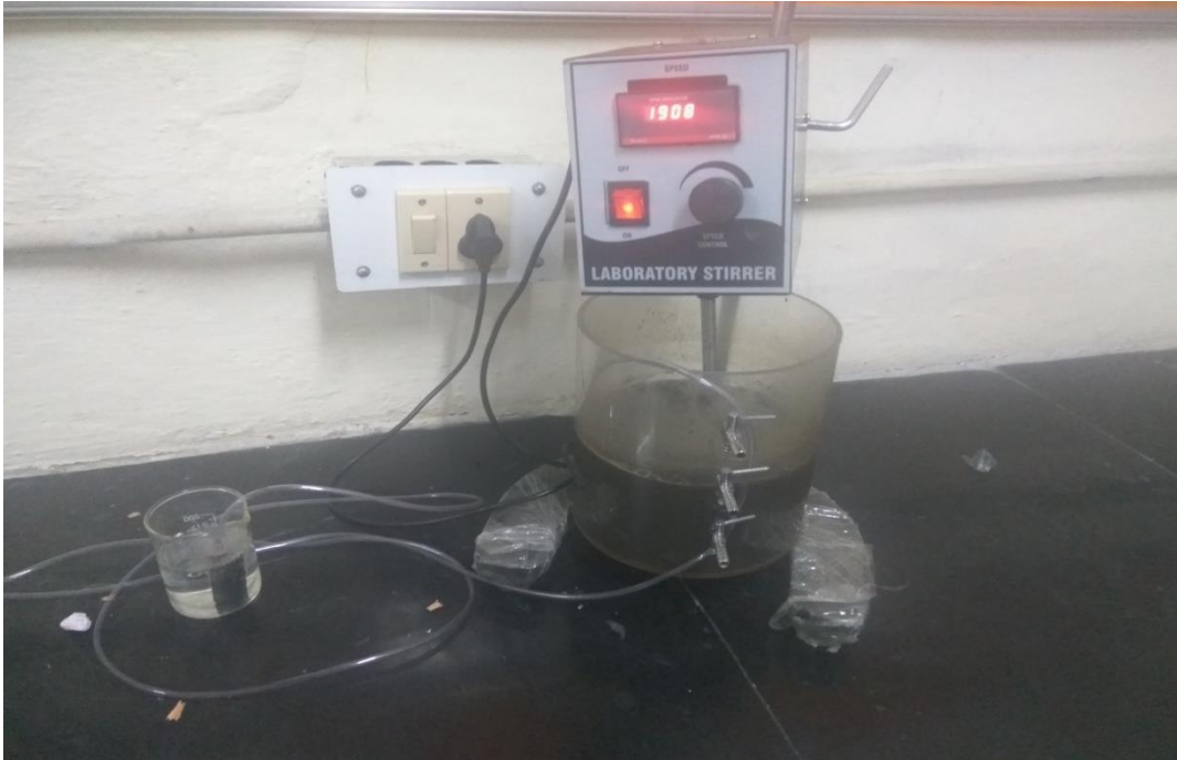
Figure A. 1 Mixing and Aeration in the Reactor
