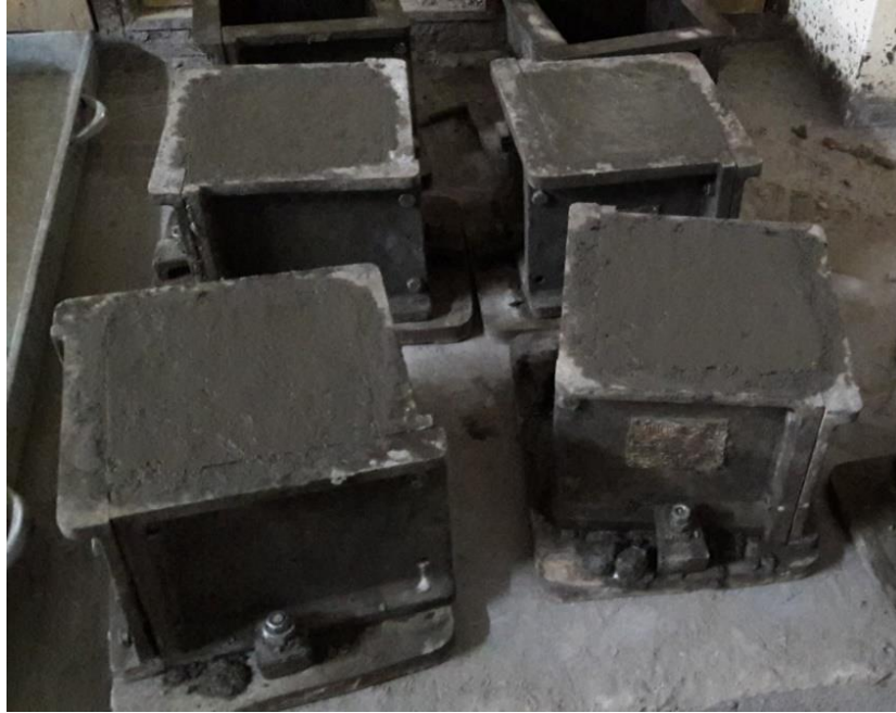
Fig 3.12. Concrete cubes in moulds
