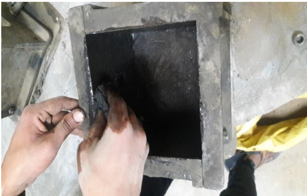
Fig 3.9. Greasing of moulds
