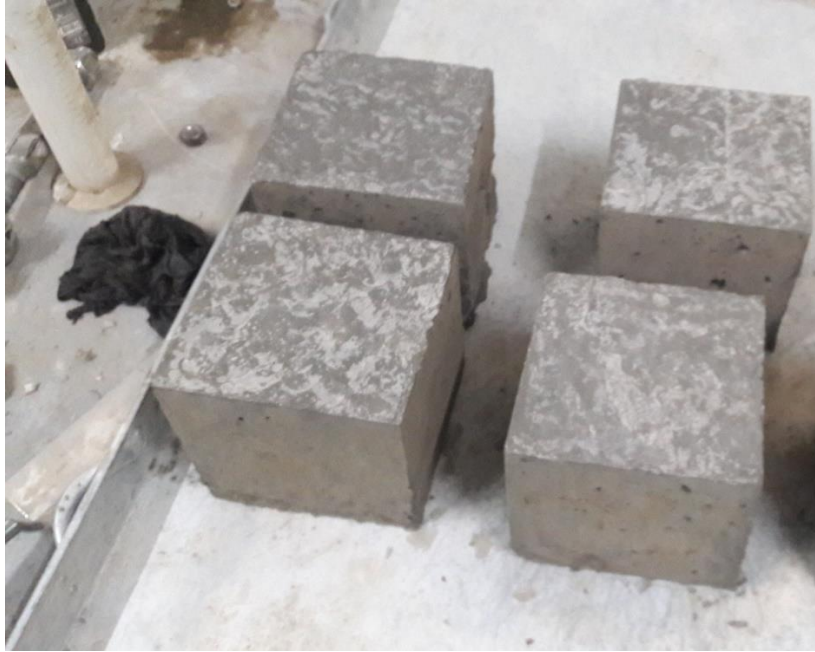
Fig 1.2 Recycled aggregate concrete cubes
