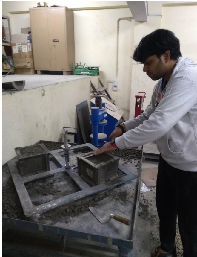
Fig 3.11. Compaction of concrete using vibratory machine
