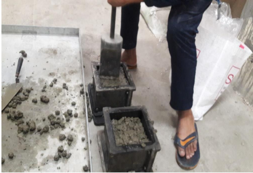
Fig 3.10. Tamping of layer by tamping rod
