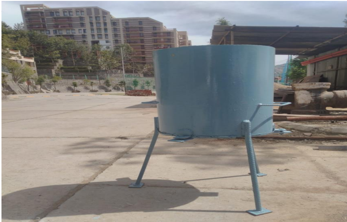
Figure 3.2 Model prepared for leachate collection
