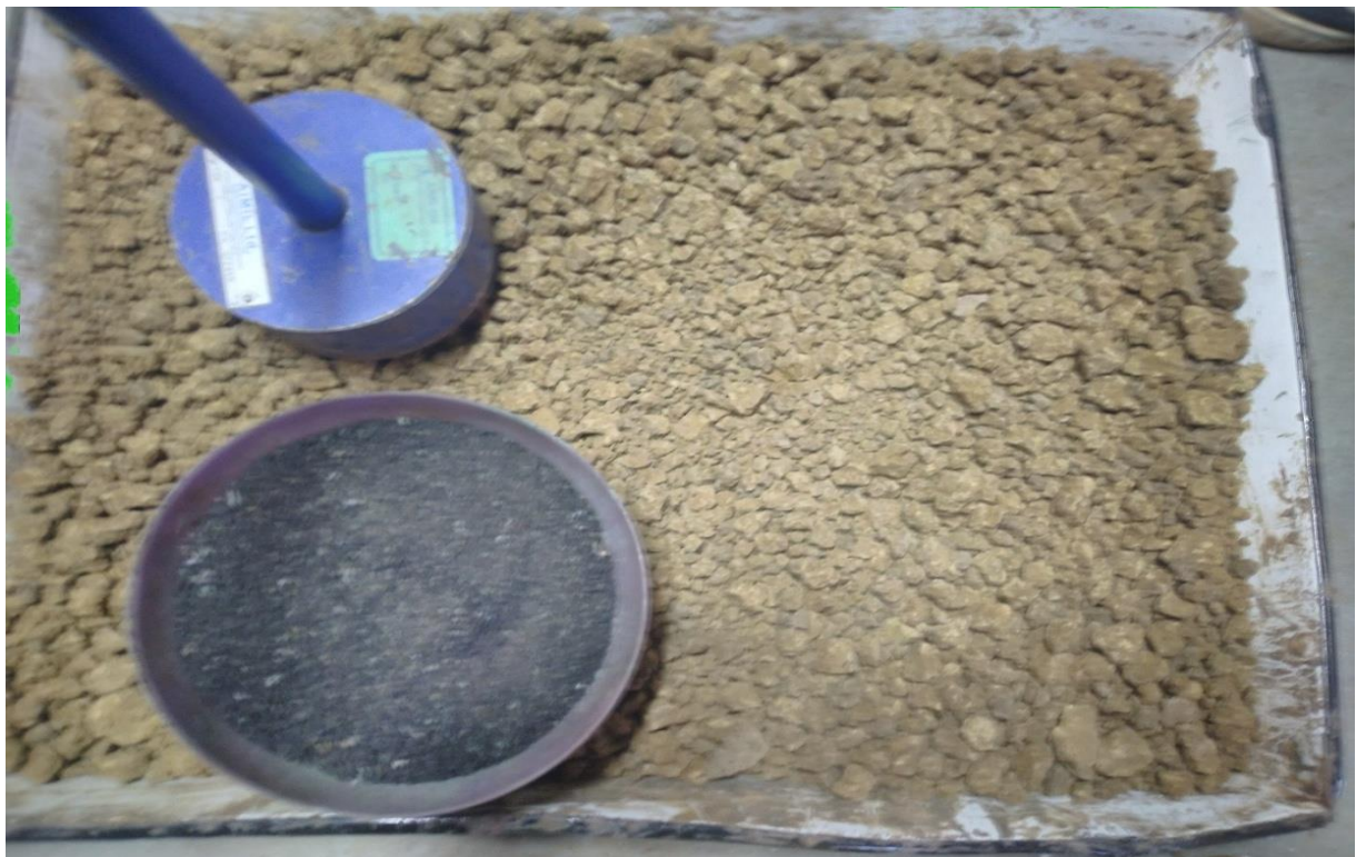
Figure 3.13 Fine crushing of the soil to remove lumps
