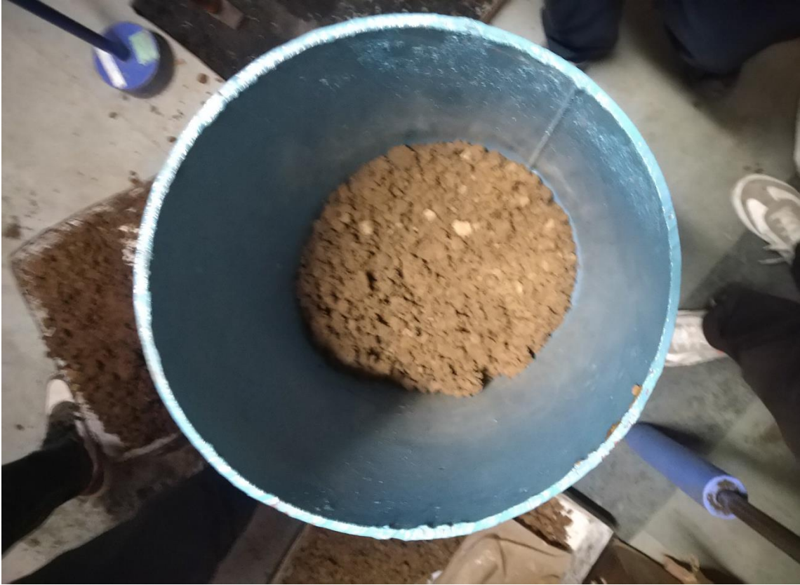
Figure 3.14 Filling of the mould with soil and leather mix
