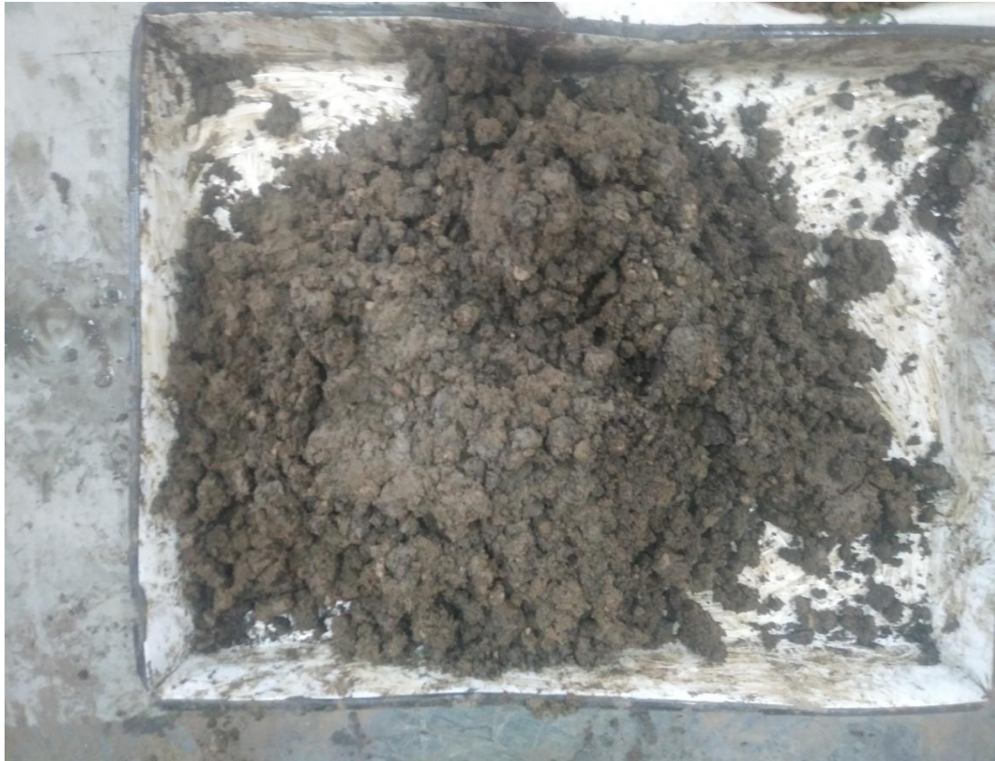
Figure 3.12 After adding water in soil mixed with leather waste
