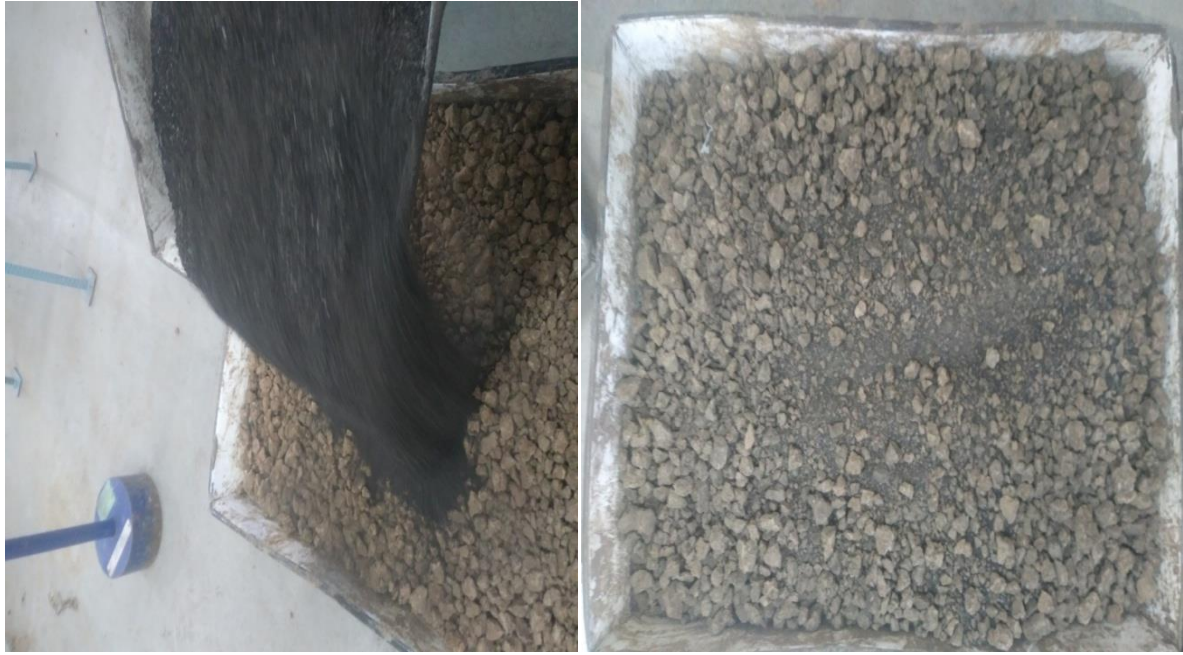
Figure 3.10 Mixing of black cotton soil with burnt leather Figure 3.11 Evenly mixed burnt leather with soil
