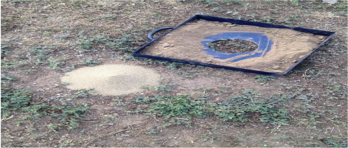
Fig.13: Sand Replacement test
